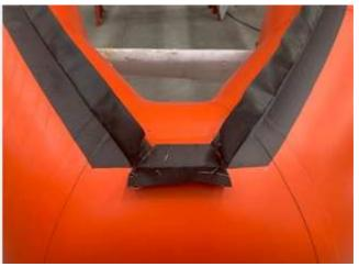
3. Replace the Tube onto the Hull and then glue the loose part to the Hull
