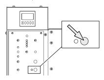
Set the sensor switch to ON.
