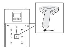
Set the chain pusher switch to ON (A). When the chain pusher starts moving forward, the chain vise is in its UNLOCKED position (C). Set the chain pusher switch to OFF (D).
