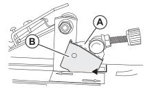
2. Use a finger to press plate B downward and forward into the "Skip tooth" position.
