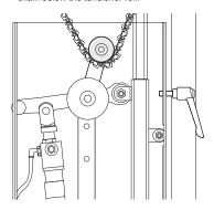
When using the lower tensioner roll, lift the tensioner arm (there is a quick release function) and place the chain below the tensioner roll.
