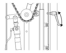
Gently press the chain with your hand to test the tension. The chain should not slacken.
