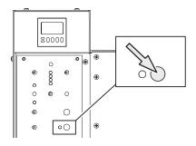
2. Set the grinding speed knob to high speed. See section 3.6.2, "Grinding speed knob".
