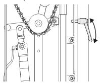
When using the upper tensioner roll, place the chain below the tensioner roll.
