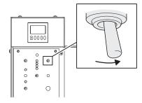
Set the chain pusher switch to ON to start the feeding of the chain and the movement of the grinding head. The sharpening will start after this
