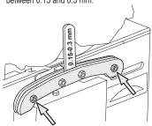
If the groove is not between 0.15 and 0.3 mm wide, turn the nut (A) in 1-1.5 turns clockwise, until the groove in the chain vise is between 0.15 and 0.3 mm.
