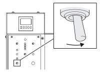
Set the grinding wheel switch to ON to start grinding motor.
