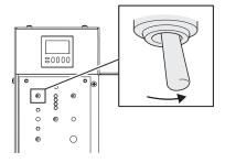
Visually make sure that the left sensor finger is pushed in by left cutters and that the right sensor finger is pushed in by right cutters.
