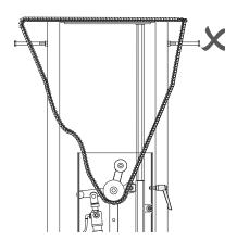
If the chain tension is too loose, repeat the procedure.
