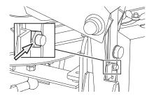
Turn the grinding head to set the desired head-tilt angle (50-70°) on the head-tilt angle scale. The default head-tilt angle is 60°.
