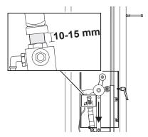
Tighten the locking handle to secure the chain.
