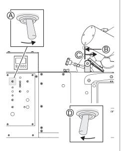
Make sure that the groove in the chain vise is approximately 2.2 mm. Insert the feeler gauge. Adjust the nuts if necessary to adjust the chain vise so the feeler gauge can slide out.
