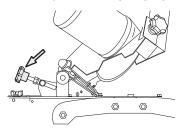
Set the chain pusher switch to OFF when the grinding head is in its uppermost position and the chain lock is not engaged.
