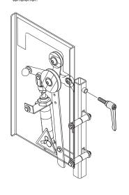
Then insert the rod through the unit and insert the bottom part of the rod onto the base of the stand
