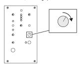
3. Press the grinding head positioning button to turn the grinding head to the left.
