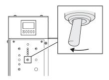
Use the hex key (provided with the machine) to loosen the top-plate angle screw up to three turns.
