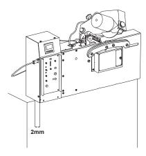
If the machines are not being used with the stand and the pneumatic tensioner, it should be used with the weight tensioner in order to provide the chain with the tension needed for grinding. The weight tensioner is available separately for purchase (see section 8, "Accessories and Spare Parts").
