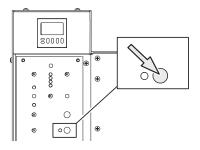
2. Set the grinding speed knob to low speed.
