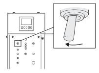
Lift the tensioner arm (quick release function) and remove the chain.
