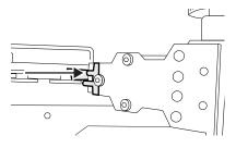
Also, visually make sure that the sensor fingers are released when the cutters move forward and no longer push the fingers in. If the fingers are not released, see section 7.3, "Issues".
