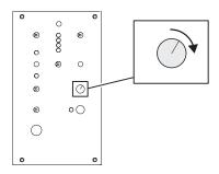
3. Set the grinding wheel switch to ON.
