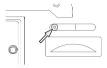
Turn the grinding head to set the desired top-plate angle (0-35°) on the top-plate angle scale. The default top-plate angle is 30°.
