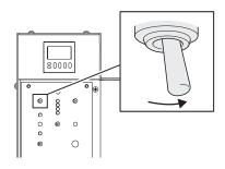
Press the reset button when the grinding head moves downward the first time. This resets the counter.
