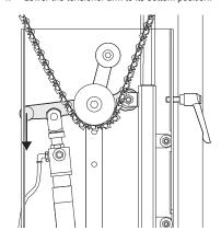
Move the tensioner downward until the chain is tightly secured in its position. There should be a gap of about 10-15 mm between the pneumatic-piston nut and pneumatic piston, where the piston should be visible.
