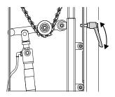
Gently press the chain with your hand to test the tension. The chain should not slacken.
