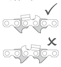
Pull the chain around by hand to make sure that it runs freely in the chain vise and does not wobble
