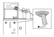
Set the chain pusher switch to ON to start the feeding of the chain and the movement of the grinding head. The sharpening will start after
