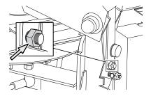
Turn the grinding head to set the desired head-tilt angle (50-90°) on the head-tilt angle scale. The default head-tilt angle is 60°.
