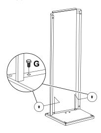
Next, attach the two side pieces to each other with provided bolts through the holes at the intersection of two pieces to create the side support piece.
