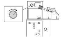
Set the grinding wheel switch to ON.
