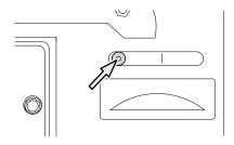
Turn the grinding head to set the desired top-plate angle (0-35°) on the top-plate angle scale. The default top-plate angle is 30°.
