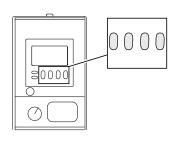
If required, press the reset button to reset the counter and start grinding again.
