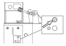
If the top-plate angles are not the same (for example 26° in the right direction and 30° in the left direction), adjust the nuts (A) a 1/2-turn at the time.
