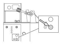
Press the grinding head positioning button to move the grinding head so that it is tilted in the correct start position for the next cutting link to be ground.
