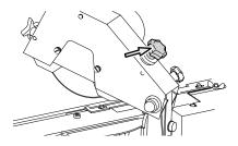
If required: Turn the chain pusher adjustment to make minor adjustments for the grinding length.
