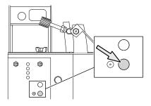
Set the grinding speed knob to medium speed.
