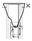
7. If the chain tension is too loose, repeat the procedure.
