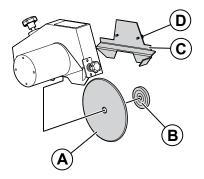
Remove the wheel attachment nut from the 3 hub.
