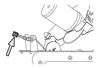
Set the chain pusher switch to OFF when the grinding head is in its uppermost position and the chain lock is not engaged.
