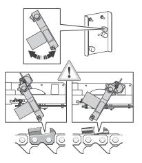
Lift the grinding head to its uppermost position.
