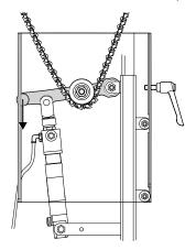
Move the tensioner downward until the chain is tightly secured in its position. There should be a gap of about 10-15 mm between the pneumatic-piston nut and pneumatic piston, where the piston should be visible.
