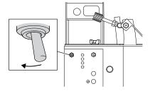
Visually make sure that the chain pusher stops its movement exactly above the rivet behind the cutting link, as illustrated in the image below.
