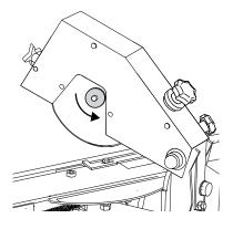
Next, insert the appropriate wheel onto the hub and, using moderate pressure with your hands. secure the wheel attachment nut to hold the wheel in place.
