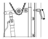
Lift the tensioner arm (there is a quick release function) and place the chain below the tensioner roll.
