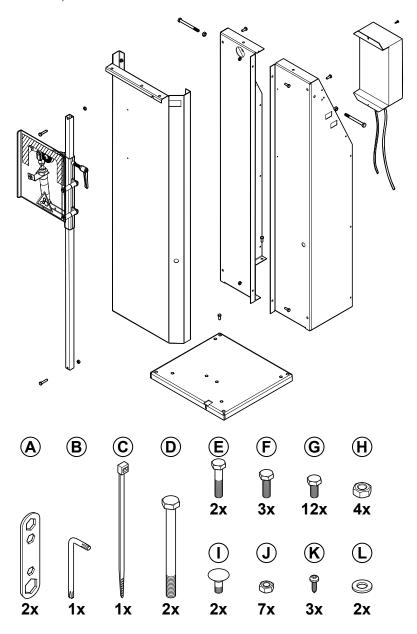
Start by placing the base piece on the floor. Place the front piece on top of the base piece by aligning the holes they have on the front right and left corners. Bolt the front piece to the base through the two holes using the provided wrench.
