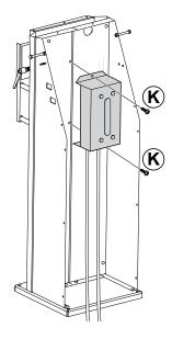
Next, place the machine on the stand. Fix it to the stand through the 3 holes located at the back of the machine with the bolts and nuts provided.
