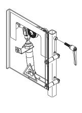
Then insert the rod through the unit and insert the bottom part of the rod onto the base of the stand
