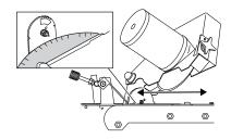
3. Tighten the head-tilt angle nut.
