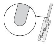
Repeat steps 4-8 until the grinding wheel profile is the same as the selected profile on the profile template.
