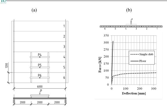
**FIGURE 2** (a) Test setup adopted by Lejeune and Niet<sup>28</sup>; (b) Experimental load displacement curves up to failure obtained from tests on the floor and on a single unit. *Source*: Adapted with permission.<sup>28</sup>
