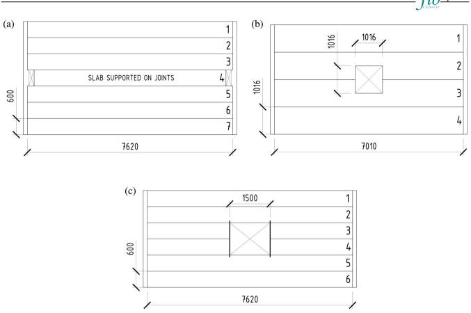
FIGURE 1 Sketch of the test setups investigated by LaGue (a, b) and Johnson and Ghadiali (c). Source: Adapted with permission.<sup>26,27</sup>
