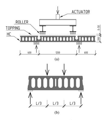
**FIGURE 7** (a) Shear tests by Hong et al.<sup>44</sup>; (b) Four-point bending test setup by Pisanty.<sup>46</sup> HC cross sections should be intended as indicative. *Source*: Adapted with permission.<sup>44,46</sup>
