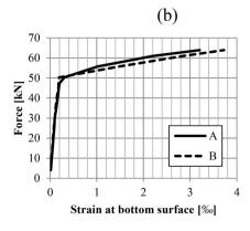
FIGURE 8 (a) Test setup of the experiments by Walraven, Huyghe and Stroband.<sup>47</sup> (b) Experimental load–strain curves measured at midspan under the load location.
