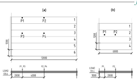
FIGURE 4 Finnish point load distribution tests: (a) 12 m long floor<sup>31</sup>; (b) 6 m long floor.<sup>32</sup> Source: Adapted with permission.<sup>31,32</sup>
