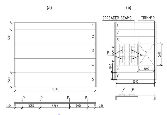
**FIGURE 3** (a) Test setup by Pfeifer and Nelson<sup>29</sup>; (b) Test setup of a floor with a large opening supported on a concrete trimmer beam.<sup>30</sup> *Source*: Adapted with permission.<sup>29,30</sup>
