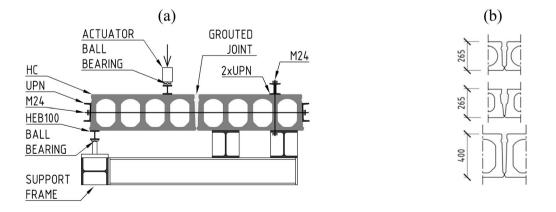
**FIGURE 6** (a) Experimental setup of the tests performed by den Uijl.<sup>44</sup> (b) Geometry of the joints considered. *Source*: Adapted with permission.<sup>44</sup>
