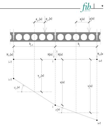
**FIGURE 11** Illustration of the equilibrium condition in a longitudinal joint.
