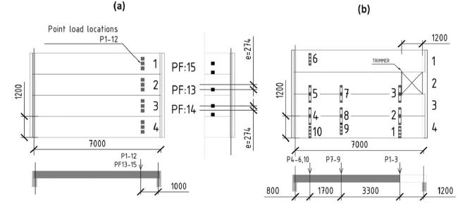
FIGURE 5 Load distribution tests<sup>33,34</sup> on (a) 400 mm floor, (b) 200 mm floor with opening. Source: Adapted with permission.<sup>33,34</sup>
