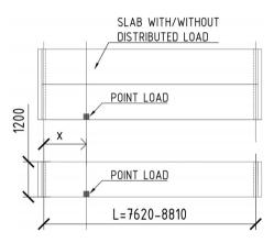
**FIGURE 10** Experiments on concentrated load capacity by Aswad and Jacques,<sup>49</sup> two-unit assemblies (top) and single unit test (bottom).
