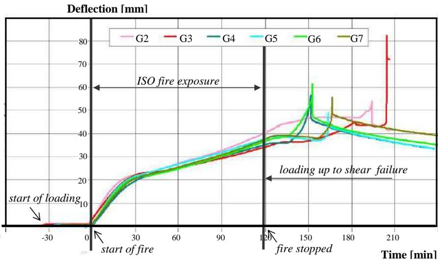
Figure 3.10.b Time – deflection diagram of fire tests G2 to G7
