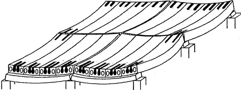
*Fig. 4.19 Recommended solution for hollow core floors with flexible supports, exposed to fire*
