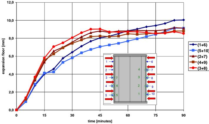
Figure 6.8. Relative displacements of floor R2 (hcs 260 mm – 100 mm topping) at centroid of underflange
