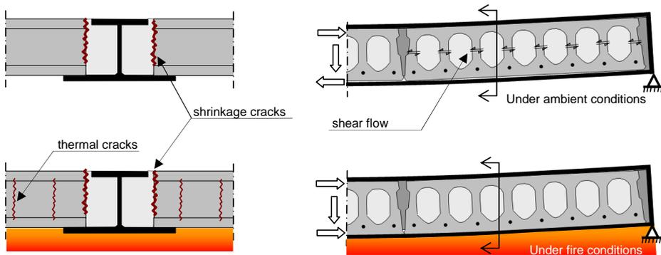
Figure 4.14. Flexible support effect at support under ambient conditions (above) and under fire conditions (under)
