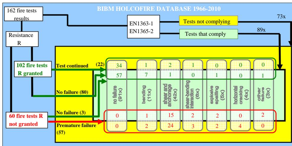
Figure 2.8. HOLCOFIRE fire test database comprising 162 fire test results on hollow cores
