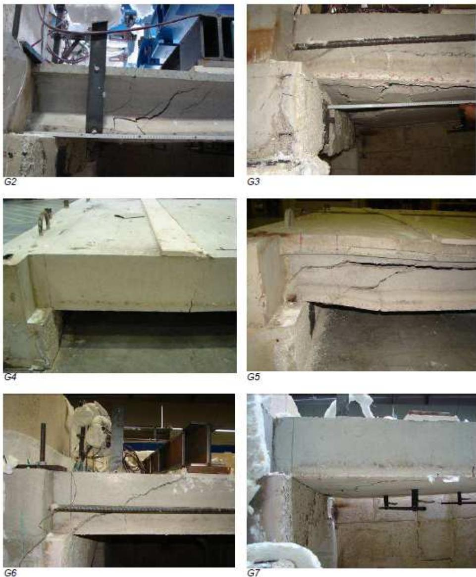
*Figure 3.11. Photos of failure cracks at the sides of the floors after further loading up to failure after the fire was stopped*
