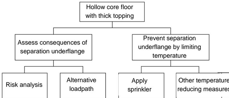
Figure 5.11. Measure “A”: proposed approach for hollow core floors with thick toppings
