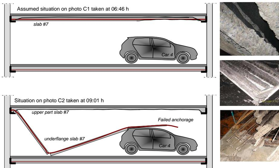
Figure 5.16. Slab #7 felt down several hours later due to anchorage failure, situations at 06:46 h and 09:01 h
