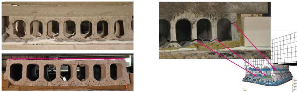
Figure 5.9. Experimental studies of part of hollow core slab with and without topping, restrained conditions and FEM
