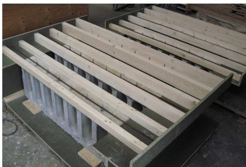
Figure 30. Production of the samples of slices of hollow core slabs
