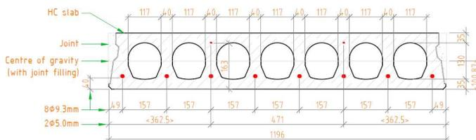
**Slipformed concrete slab**
