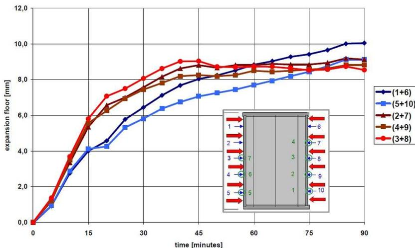
Figure 7.23. Measured horizontal transverse expansion of test R2
