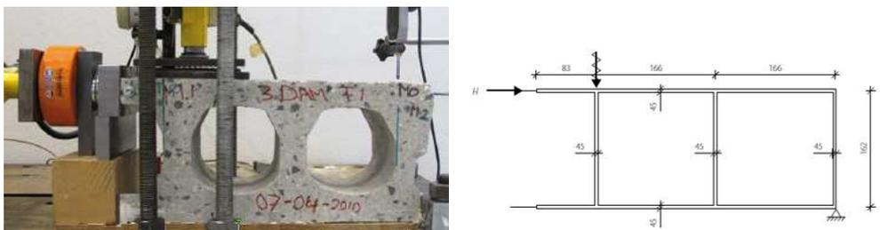
Figure 5.10. Numerical studies with simple truss analysis, shear stiffness validated with experiment
