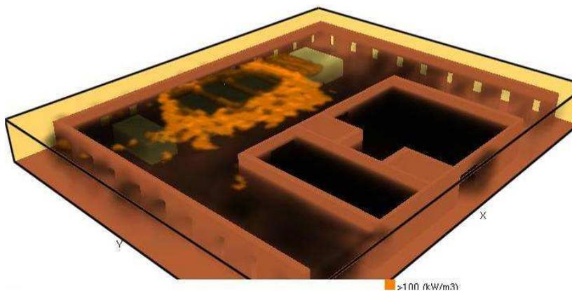
Figure 5.12. Geometry Parking Rotterdam and HRRPUV plus smoke snapshots at 30 minutes simulation in fire scenario 1 [5.31]
