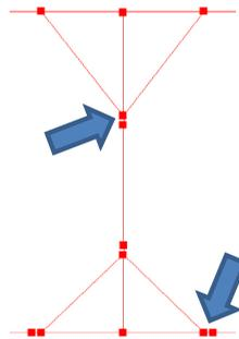
Figure 7.14. Cracking rods at the end of flange and web mid rods
