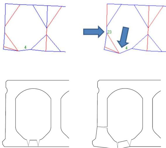
Figure 7.27. Release of the under flange by click-clack effect as shown by frame model (above) and sketched in a cross-section (below)
