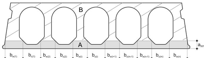
Figure 2.2. Position of line  $a_{50\%}$  and area A where solid slab temperatures may be assumed (grey) and area B for linear interpolation (hatched)
