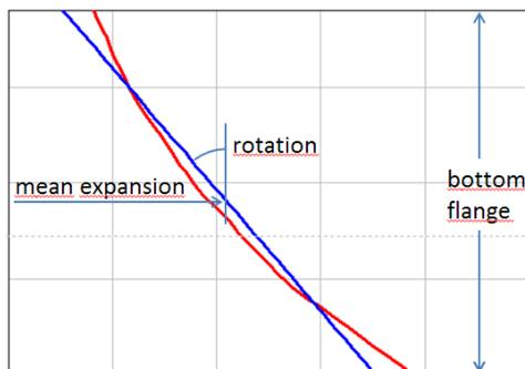
Figure 7.11. Average expansion and rotation of the under flange due to temperature
