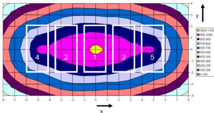
Figure 5.7. Maximum occurring temperatures as a function of location based on fire scenario 1, cars are visualized [5.3]
