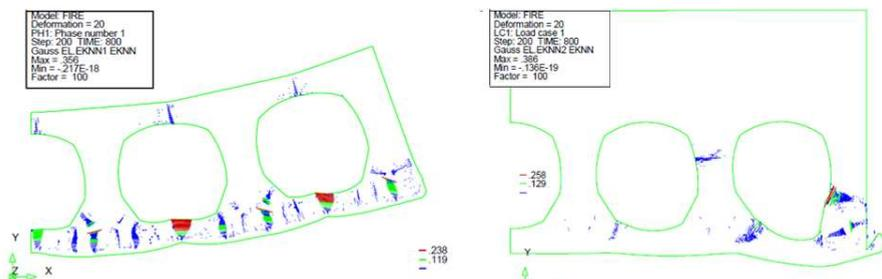
Figure 5.5. FEM simulation of hollow core with topping; unrestrained (variant 1, left) and fully restrained with thick topping (variant 2, right) [5.2]
