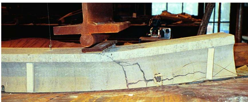
Figure 2.11. Fire test H122: Shear and anchorage failure; shear crack visible at shear span and crack at level of strands
