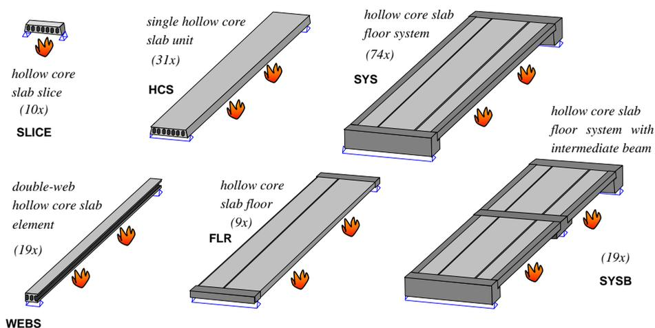
Figure 2.7. Test set-up lay-outs in database (162x); slices, double-web elements, single slabs, floors, and systems
