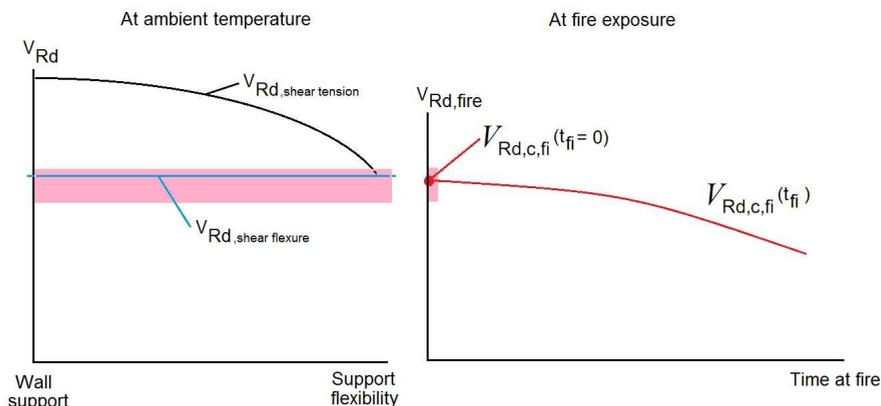
Figure 4.15. Ambient shear resistance (left) and shear resistance under fire (right)
