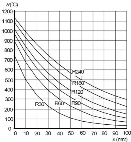
Figure 7.9. Temperature profiles for slabs (Annex A of EN 1992-1-2)
