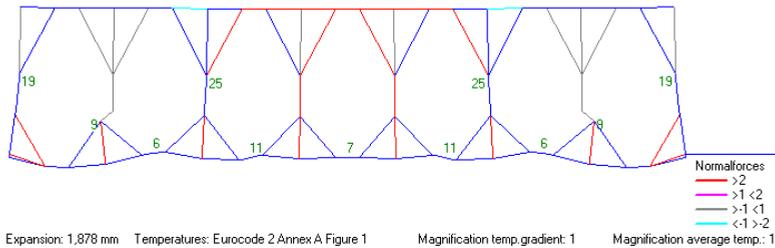
Figure 7.26. Result of analysis of blocked cross-section HC260/7
