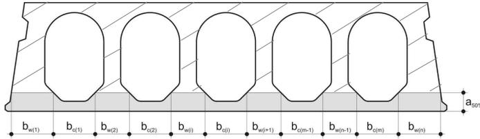
Figure 3.2. Area where solid slab temperatures may be assumed (grey area)
