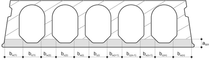
Figure 4.16. Area where solid slab temperatures may be assumed (grey area).
