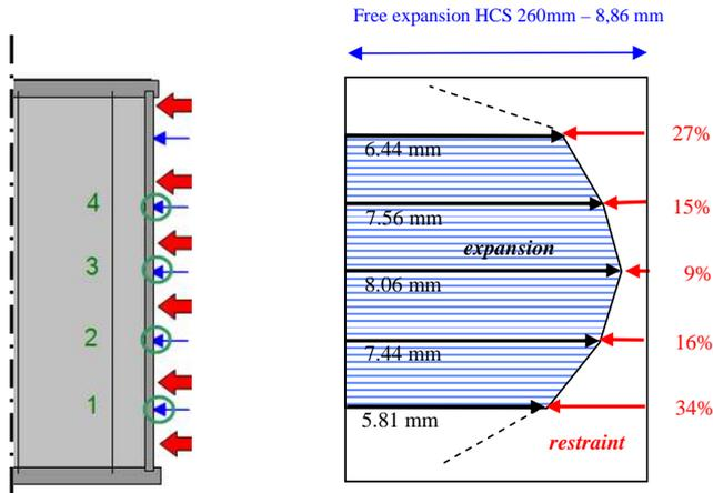
Figure 6.9. Expansion of the floor R2 at 30 minutes, and calculated restraints at centroid of underflange
