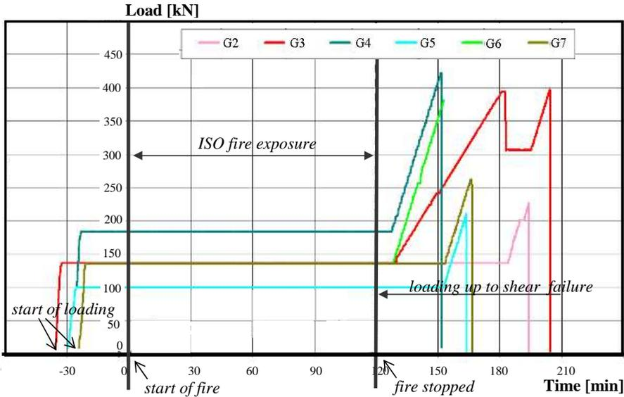
Figure 3.10.a Load – time diagram of fire tests G2 to G7
