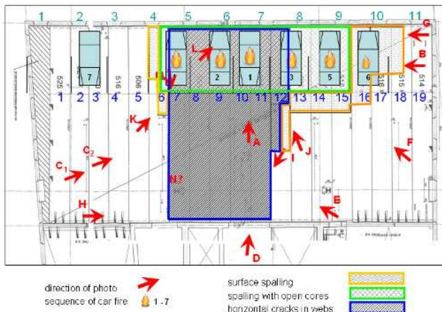
Figure 5.8. Plan overview of level 2 of parking garage with location of cars on floor and damage on the ceiling
