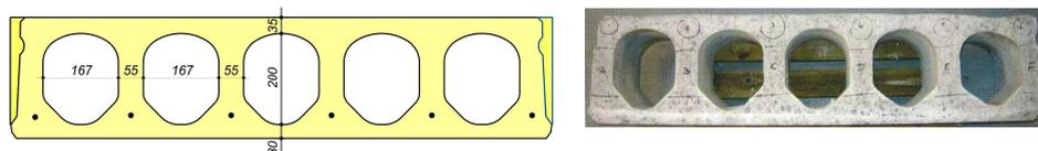
Figure 3.5. Hollow core cross section with depth 265 mm and 6 strands Ø12.5 at 50 mm axis distance
