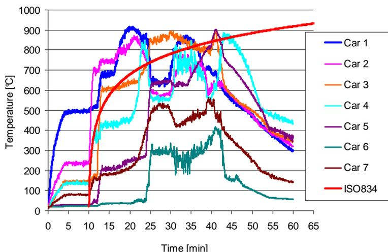
Figure 5.13. Evolution in time of the gas temperature above car 1 to car 7 and ISO 834 curve [5.31]
