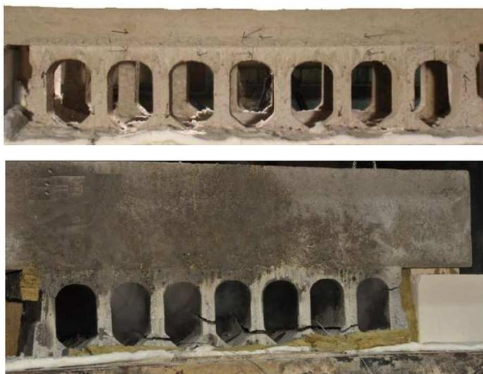
*Figure 7.4. Fire tests on small samples of hollow core in The Netherlands. Up: Slices with a structural topping. Down: free part of hollow core 1.20x1.20 m<sup>2</sup> with extreme thick topping of 300 mm*
