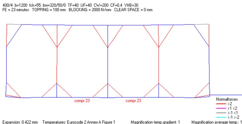
Figure 7.17. Example of frame analysis with compression failure at the soffit
