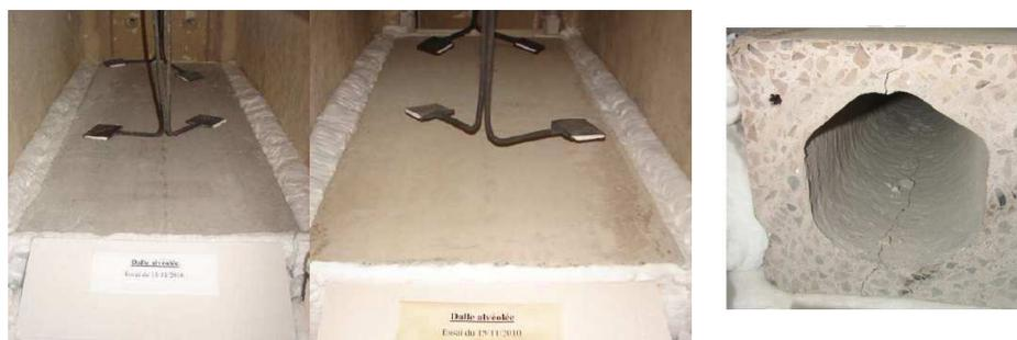
Figure 3.8. Specimen G1: before test (left) and after 2 hour fire test (middle). Vertical cracks in core after one day (right) (Note that slab was turned up-side-down in test so the soffit was facing upwards)
