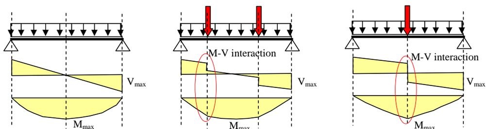
Figure 2.14. Shear-bending interaction in fire tests due to use of point loads in experiments
