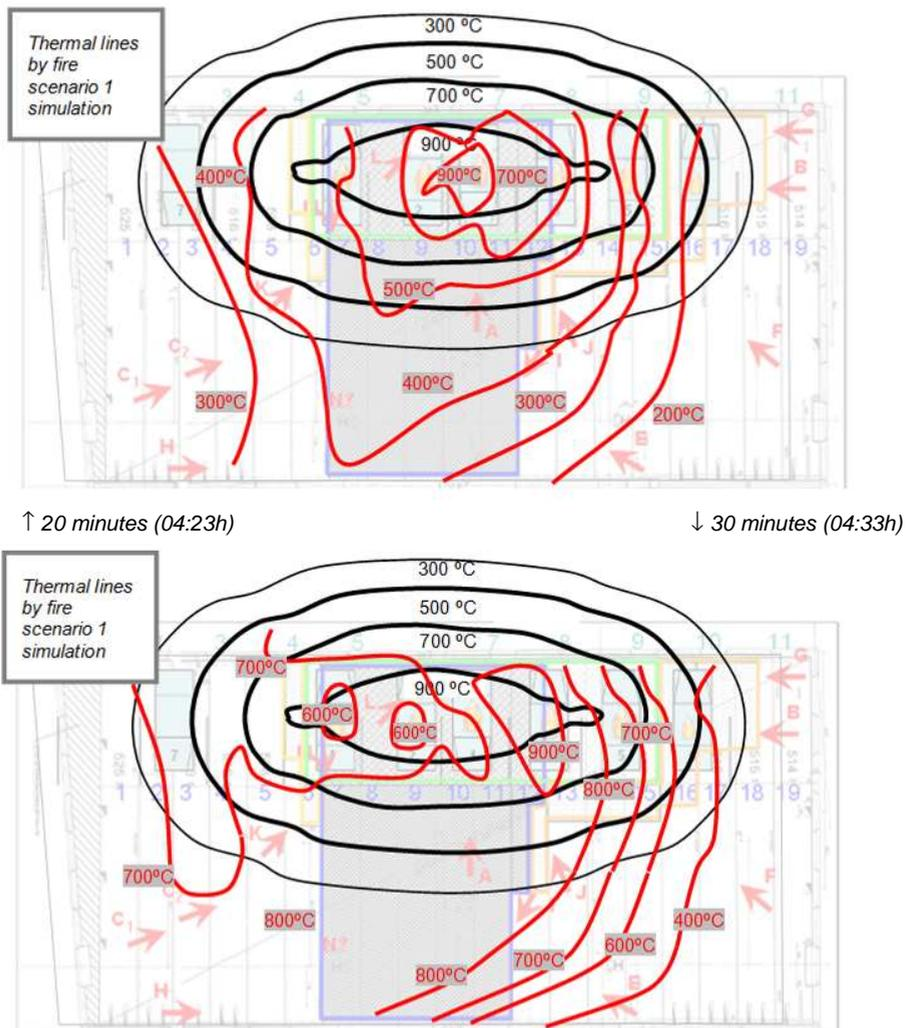
Figure 5.14. Fire scenario 1 as calculated by CaPaFi [5.1] (black lines – thermocouple temperature) and as calculated by FDS5 after 20 and 30 minutes as shown in Smokeview (red lines – gas temperature) plotted on floor plan [5.31]
