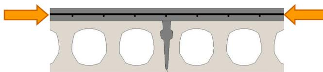
Figure 7.22. Direct blocking effect of a structural topping
