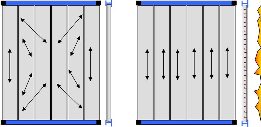
Figure 4.12. Under ambient conditions in stiff floor field the load is distributed towards stiff columns (left), while under fire conditions when webs are cracked the floor is less stiff and load is distributed in longitudinal direction (right)
