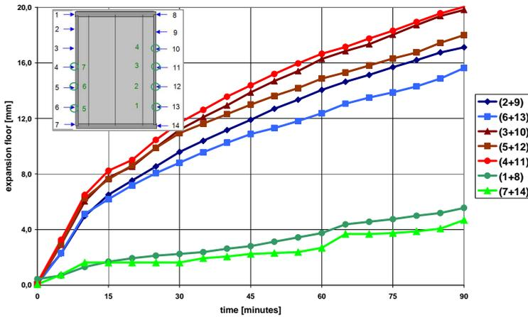
Figure 6.10. Relative displacements of floor R3 (hcs 200 mm – 50/70 mm topping) at centroid of underflange
