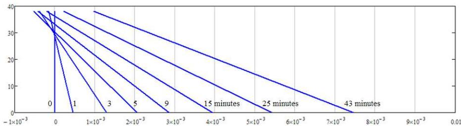
Figure 7.13. Strain of under flange following calculated values of ISO 834 fire curve
