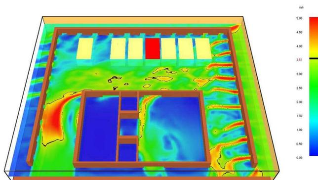
*Slice wind velocity [m/s] snapshot at the beginning of simulation Fire / burner*
