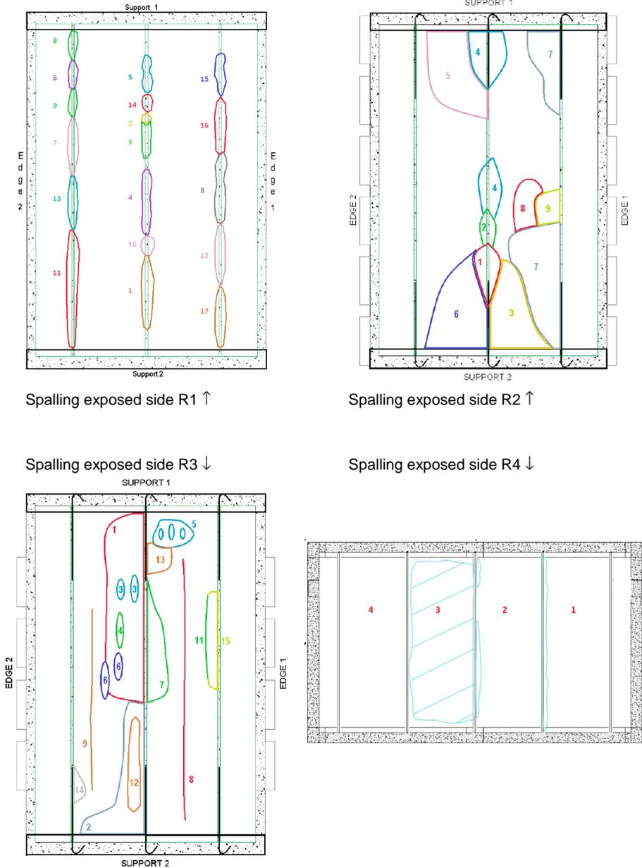
Figure 6.7. Sketches of spalling at the soffit of the tested floors registered the day after the fire test was executed
