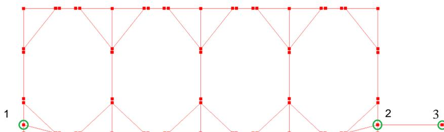
Figure 7.15. Additional rod (between node 2 and 3) representing the blocking spring
