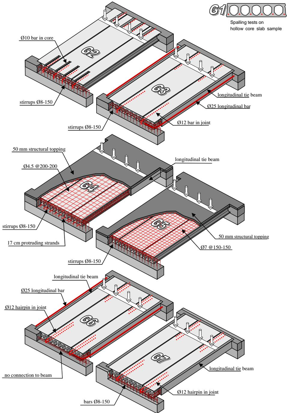
Figure 3.4. HOLCOFIRE series G – overview of floor geometries G1 to G7
