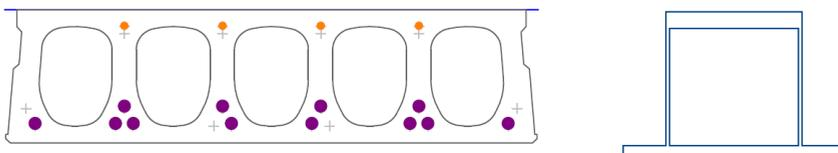
Figure 4.18 Cross sections of hollow core 315 mm and THQ320 beam
