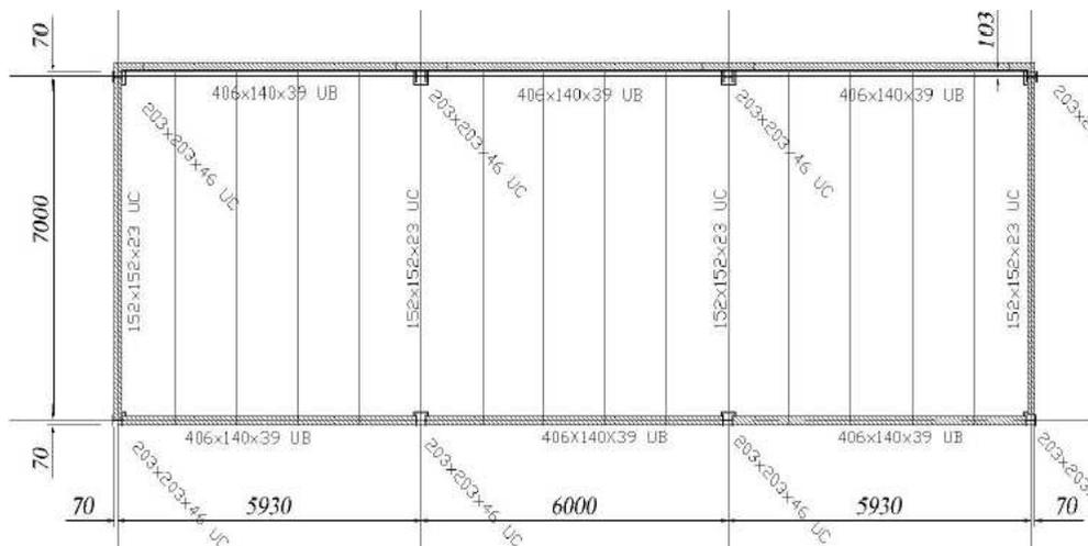
Figure 4.6. Plan of BRE full scale fire test in Cardington [4.14]
