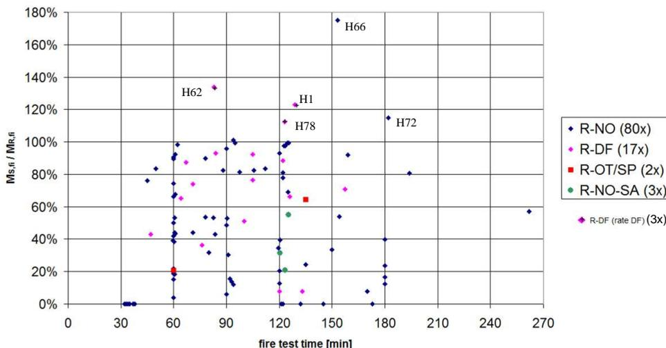
Figure 2.10. Bending moment over bending capacity versus time of 102 tests that did not fail in bending
