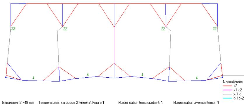
Figure 7.16. Example output of frame analysis with web cracking; in the outermost web a bending crack occurs at 22'; in the 2<sup>nd</sup> web horizontal web cracking initiates at 22'
