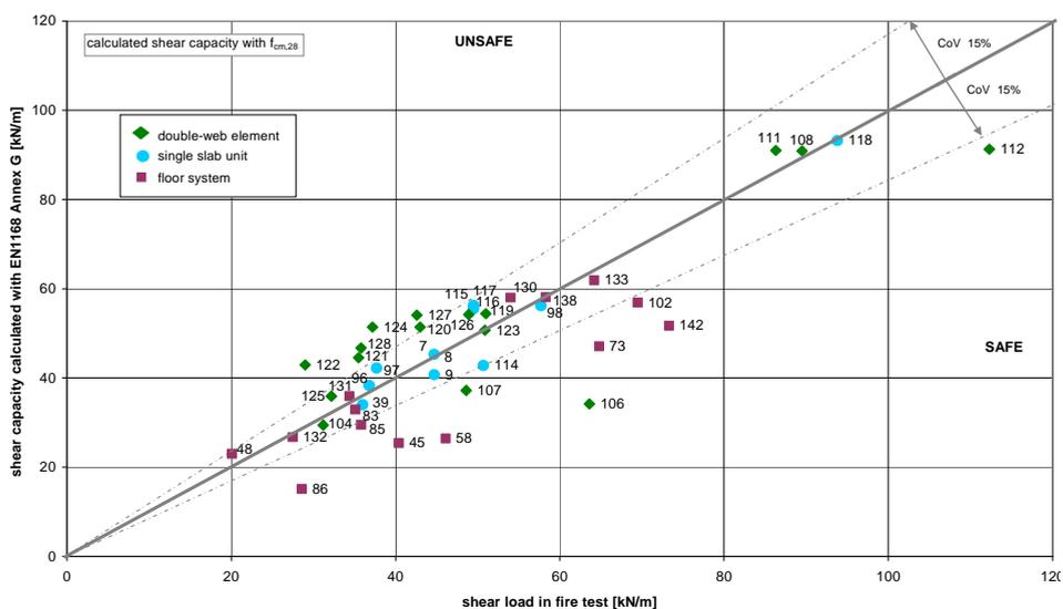
Figure 2.12. Relation shear capacity from fire test versus shear capacity calculated with EN1168 Annex G
