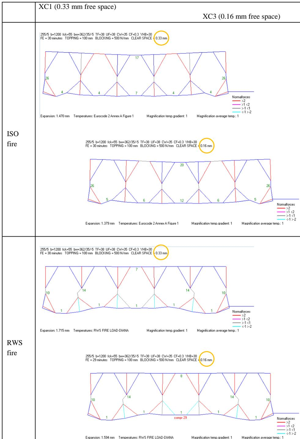
Figure 7.28. Analysis with different fire curves and different free-spacings depending of the humidity grade
