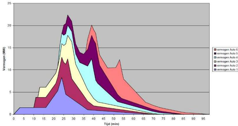
Figure 5.6. Total calculated fire power range in fire scenario 1 with 6 cars subsequently on fire [5.1]
