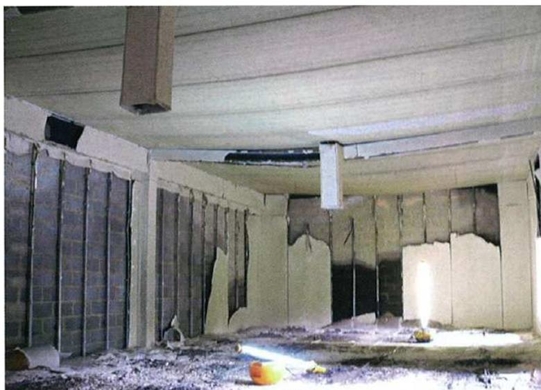
Figure 4.7. View within the compartment after the fire of the first test [4.14]
