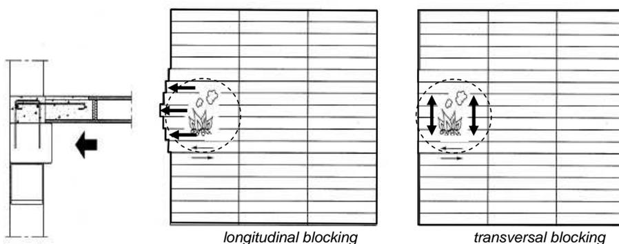
*Figure 6.1 Blocking of the thermal expansion of a floor by structural topping and surrounding structure*
