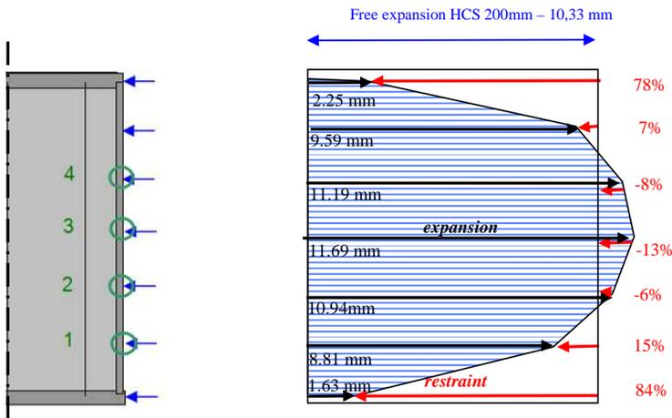
Figure 6.11. Expansion of the floor R3 at 30 minutes and calculated restraints at centroid of underflange
