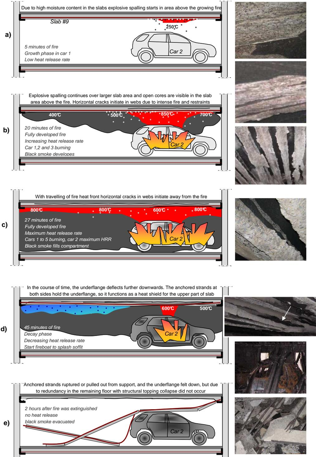
Figure 5.15 Successive phases during the Rotterdam fire of slab #9 above car 2 (KIA Sportage) (note that photos on right-hand side are meant to be illustrative and are selected from other locations)
