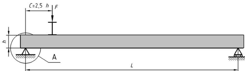
Figure 3.6. Loading scheme of slabs according to EN1168:2005+A2:2009 Annex J
