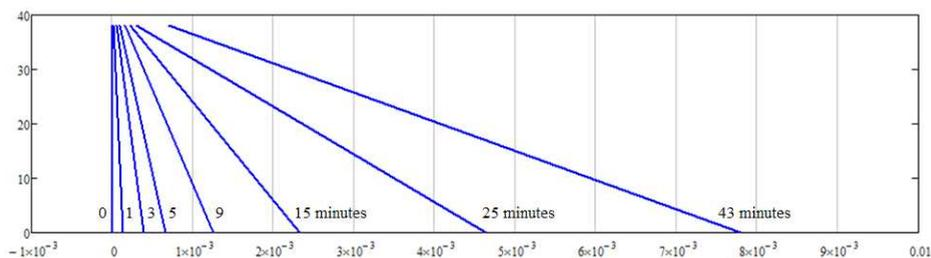
Figure 7.12. Strain of under flange at different times of fire expose with interpolated values from Annex A of EN 1992-1-2
