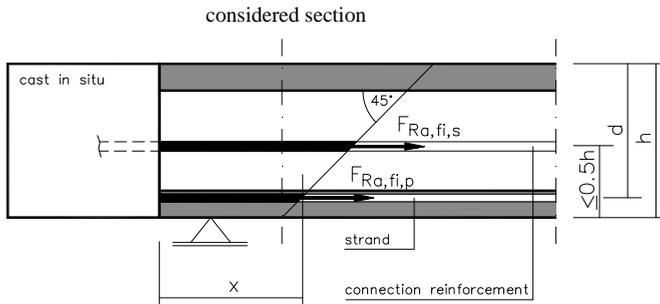
Figure 4.17. Model for calculating shear and anchorage resistance (example without protruding strands)
