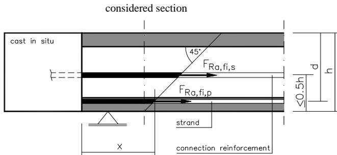
Figure 3.3. Model for calculating shear and anchorage resistance (example without protruding strands)
