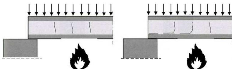
Figure 3.1. Thermal cracking due to thermal stresses (left) and cracking due to shear stresses (right)
