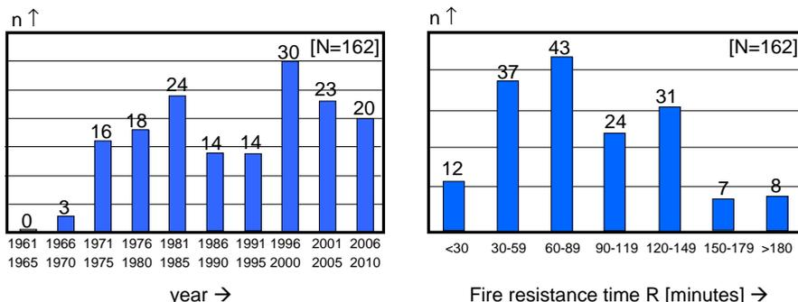
Figure 2.5. Holcofire database; division of fire test results over years, and fire resistance time reached in fire tests
