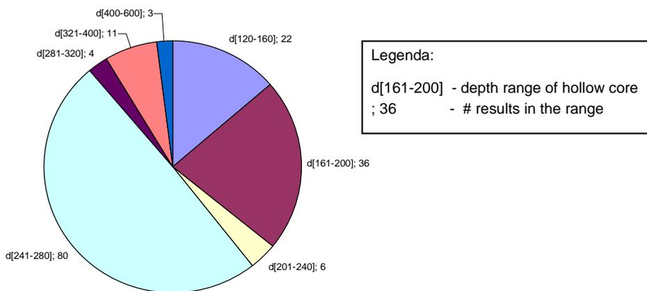
Figure 2.6. Holcofire database; depths [mm] of hollow cores used in fire tests
