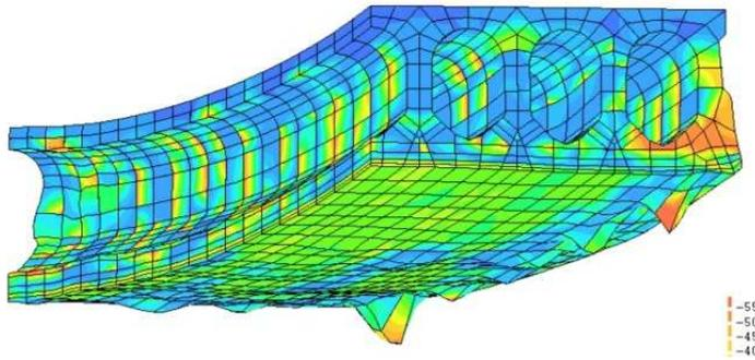
Figure 7.5. Graphical result of 3D FEM analysis with DIANA
