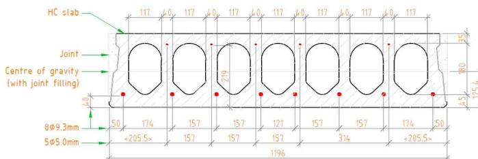
**Slipformed concrete slab**
