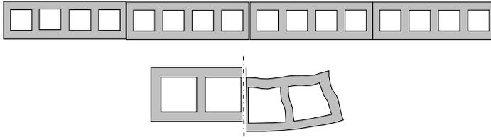
Figure 4.10 Idealized cross-section of a hollow core floor subjected to fire; initial state (left) and deformed state due to thermal expansion of the bottom flange (right)
