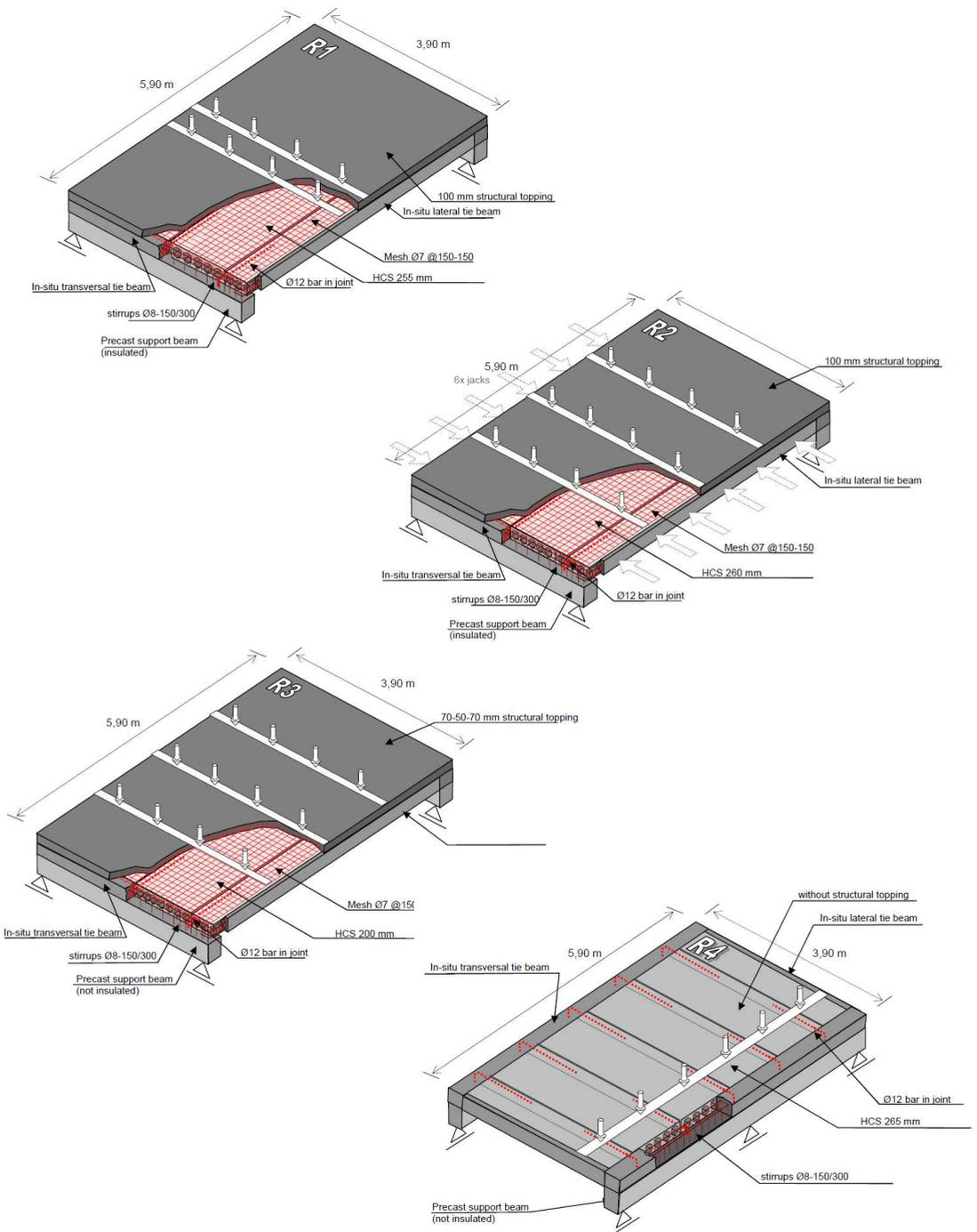
Figure 6.2 HOLCOFIRE series R – Overview of floor geometries R1 to R4
