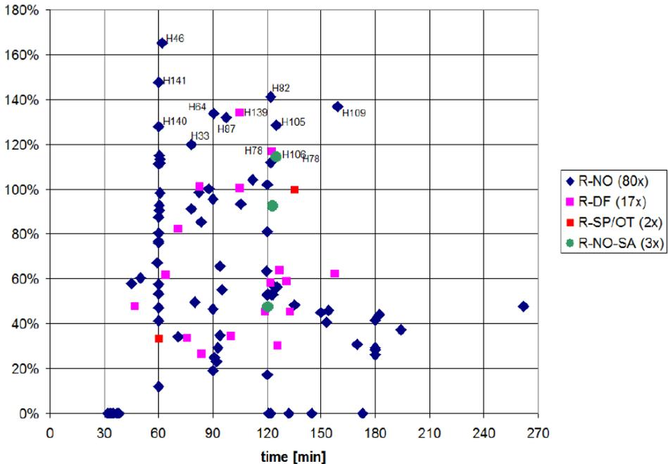
Figure 2.13. Shear load over shear capacity versus time of fire tests in which R was granted of 102 tests
