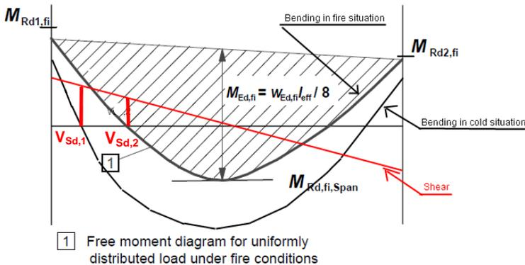
Figure 4.11. EN1992-1-2 Figure E.1 indicating positioning of free bending moment under fire, and additionally showing the reduction of shear force at point of zero moment ( $V_{Sd,1} \rightarrow V_{Sd,2}$ )
