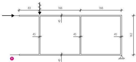
Figure 7.3. Simple framework validated on shear test on cold cross-section
