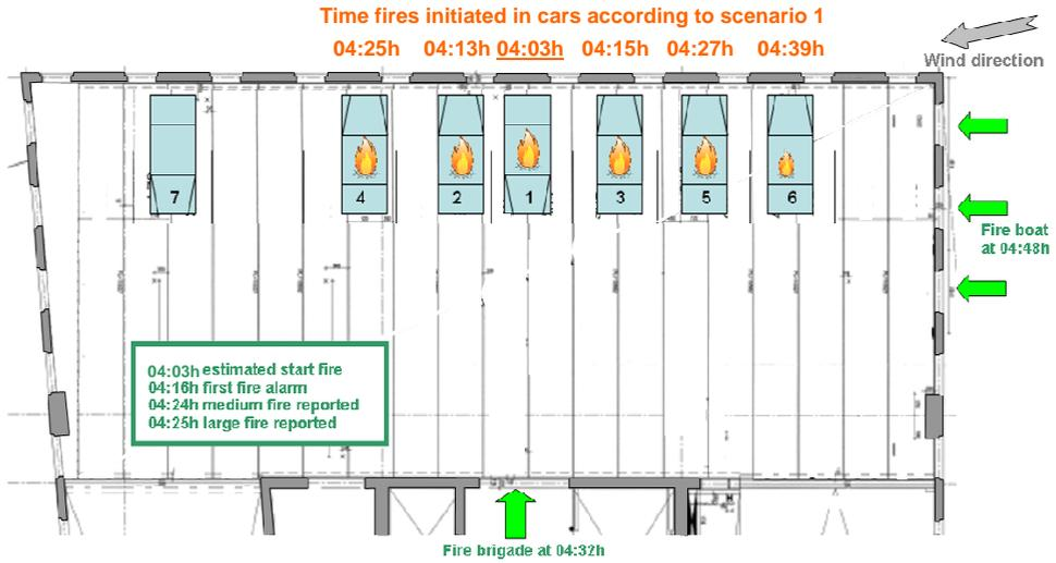
Figure 5.2. Plan overview of level 2 of parking garage with location of cars on floor and fire sequence
