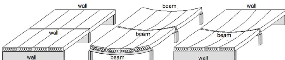
Figure 4.2. Rigid support (left); flexible supports without torsion (m) and with torsion (right) [4.5]
