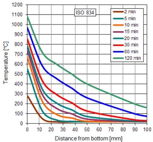
Figure 7.10. Temperature profile calculated with ISO 834 fire curve
