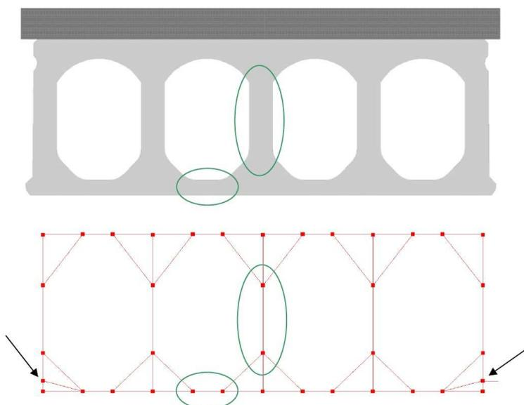
*Figure 7.7. Node and rod model of hollow core cross-section*
