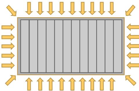
Figure 7.20. The surrounding structure induces blocking effects
