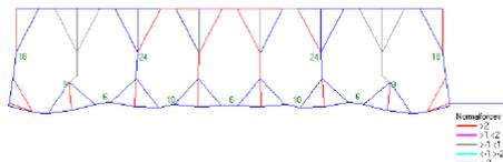
Expansion: 1.880 mm Temperature: Eurocode 2 Annex A Figure 1 Magnification temp.gradient: 1 Magnification average temp.: 1
