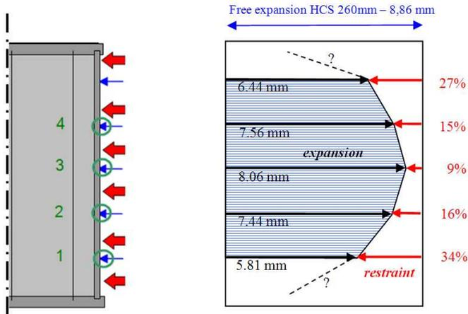
Figure 7.25. Expected restraint on base of measured expansion of the bottom flange
