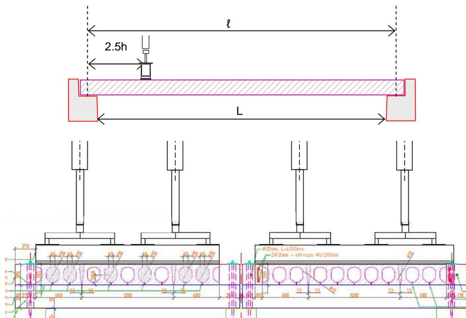
Figure 3.9. Loading scheme of slabs in fire test series G of G2/G3– longitudinal schematic view (up) and cross sectional view (down)
