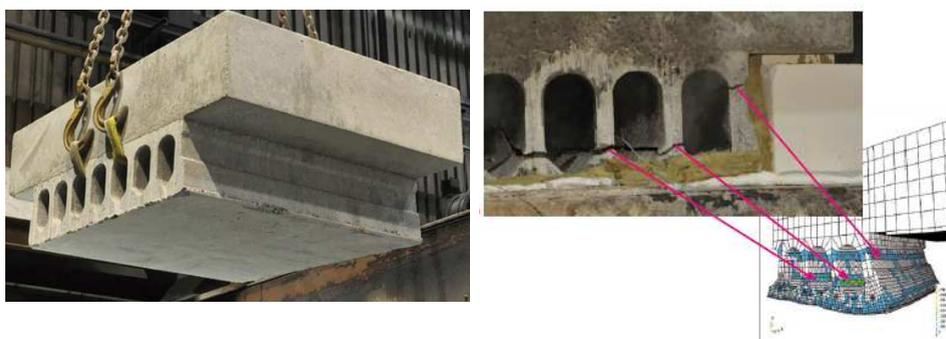
Figure 2.17. Fire test H153 with 300 mm topping and horizontal cracks through the webs
