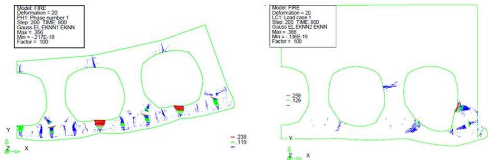
Figure 7.2. FEM simulation of hollow core with topping; unrestraint (left) and fully restraint with thick topping (right) [7.4]
