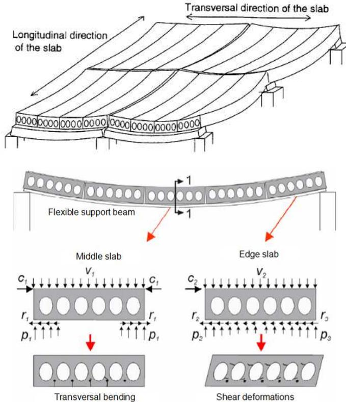
Figure 4.3. Effect of flexible supports on the hollow core slab at two positions [4.17]
