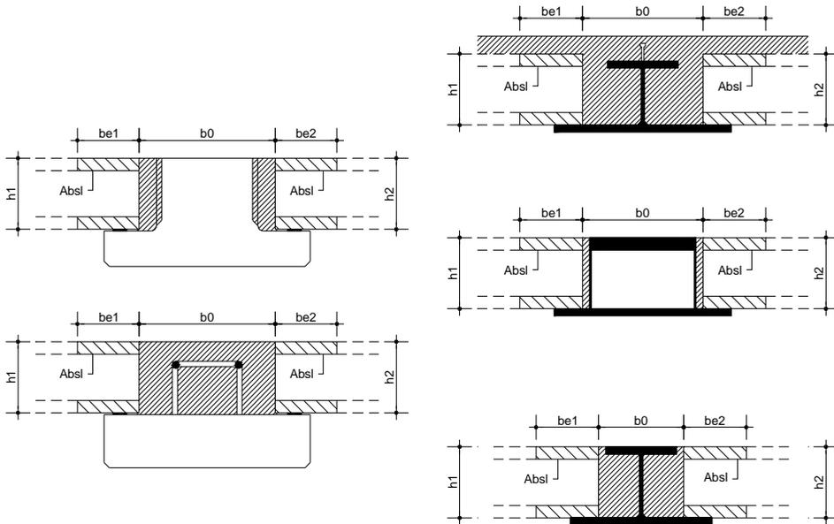
Figure 4.1. Slim floor structure with hollow core slabs (up) [4.17]; various types of slender concrete and steel beams (down) [4.4]
