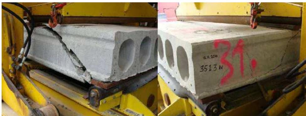
Figure 3.7. Shear tension failure crack at ambient temperature in slab #31 at both sides
