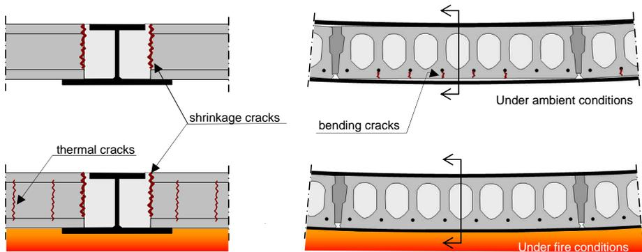
Figure 4.13. Flexible support effect at midspan under ambient conditions (above) and under fire conditions (under)
