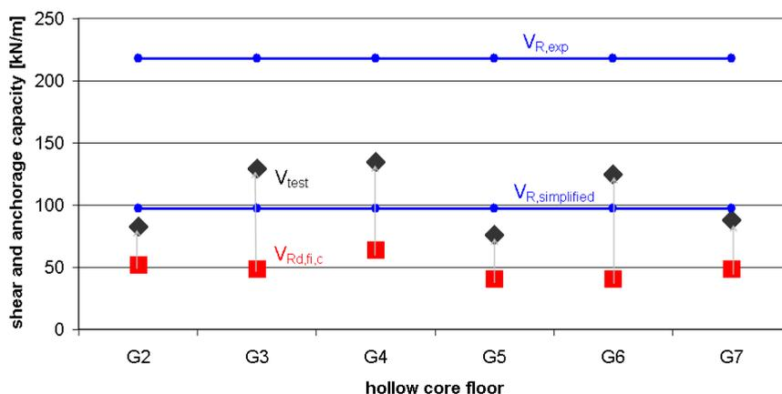
Figure 3.12. Shear capacity during fire test ( $V_{Rd,fi,c}$ ) and peak shear capacity ( $V_{test}$ ) compared to ambient shear capacity ( $V_{R,exp}$ )
