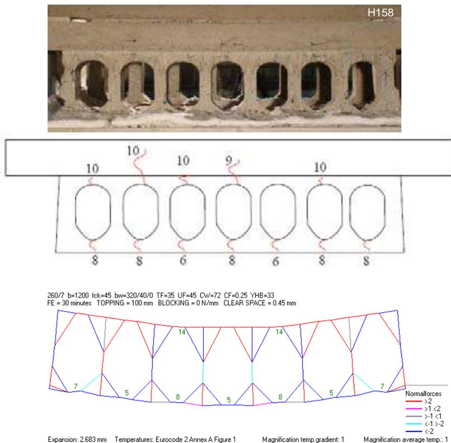
Figure 7.18. Comparison of fire test result of a slice of hollow core and topping with the frame model
