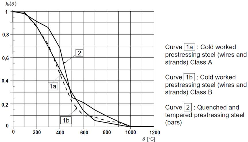
Figure 2.4. EN1992-1-2 Figure 4.3: coefficient  $k_p(\theta)$  allowing for decrease of characteristic strength ( $\beta f_{pk}$ ) of prestressing steel
