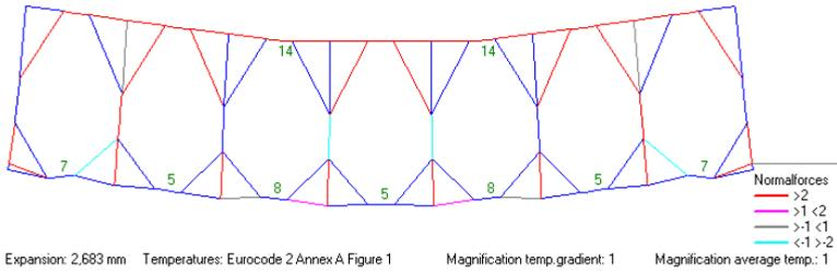
Figure 7.24. Result of analysis of free cross-section HC260/7
