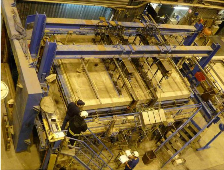
Figure 4.8. Top view of flexible support test by Peikko with Deltabeam [4.15]
