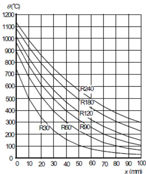
Figure 2.3. EN1992-1-2 Annex A Figure A.2: temperature  $\theta$  at depth  $x$  in slab
