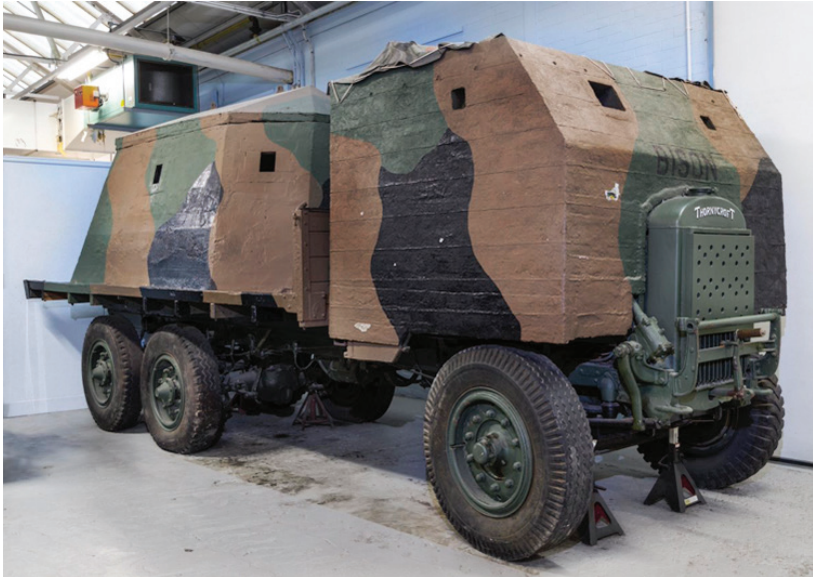
Figure 5 - "Bison" mobile pillbox, used by the Home Guard during the Second World War, with a fighting compartment protected by a layer of concrete. This example (with unoriginal chassis) is situated at the Tank Museum, Bovington, UK.
