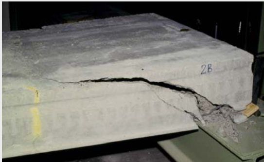
Web shear tension failure
