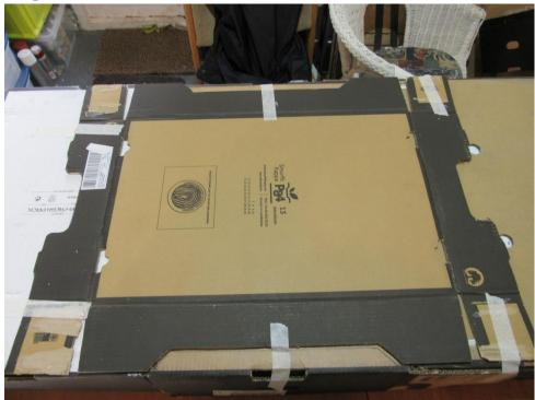
Open out and completely flatten another box and glue this in place on the underside to overlap and reinforce both central joints. Don't cut any of this box away, unless it protrudes beyond the sides of the baseboard.
