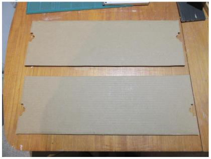
Cut the bases out of 3 of the other boxes (not the ones used for the main structure). Cut one of these bases in half so that laminating on top of the polystyrene sheet will avoid coinciding with the joints at the bottom of the main structure.
