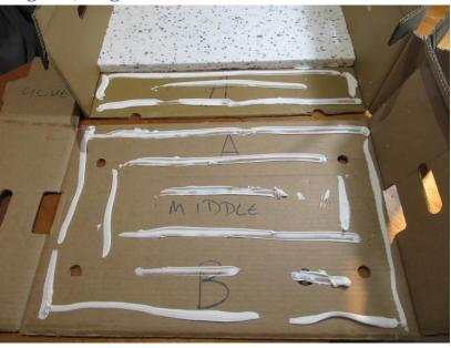
Gluing 2 boxes ready for installing the polystyrene sheet. When you install the polystyrene sheet, make sure you also run a bead of glue along the edge of the sheet where it adjoins the cardboard structure, for extra rigidity. Hold the sides more or less vertical with masking tape or string whilst the glue sets to help them stay upright.
