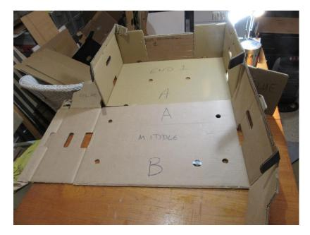
Glue the end flaps and clamp to the inside wall of the next box(es).
