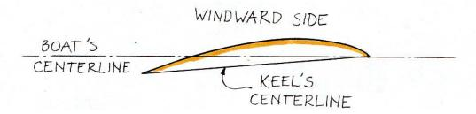
The rear portion of the keel is then carried out as a flap and the leeward side is designed as a mirror-image of first keel, then flap:
