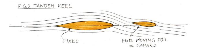
*Nippon* sported a slightly different setup in the form of a fixed main keel carrying the ballast bulb and a canard, much like a forward rudder, ahead of this. One object was to break the tip vortex up into smaller, and less retarding, portions (the wings of monokeels serve the same purpose, among others). Between each round robin series they altered the relative positions and sizes of their foils but never really found the boatspeed to match *Il Moro* and *NZ IV*.
