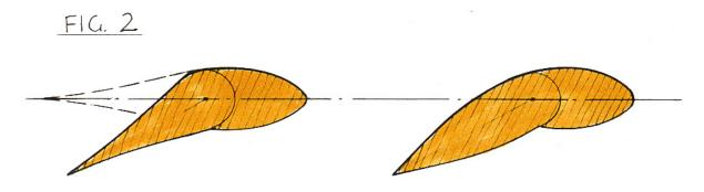
The figure shows two unlikely keel sections with much exaggerated trim tabs, or flaps, set at extreme angles. With the ordinary section, you will have an impossible stall situation caused by an abrupt change of hydrodynamic pressure at the flap joint.
