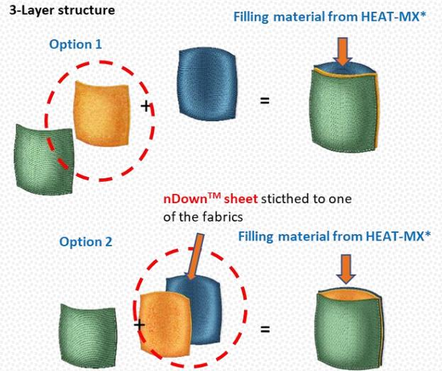
\* HMX-VN, HMX-VNBD3 or HMX-VNRD7 used as filling material
