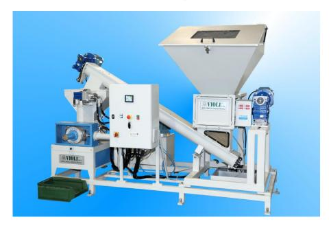
The plant is composed by a shredder suitable for the necessary production and by a hydraulic compactor mod. **VM/CTA0.** The **VM/CTAR0-01** allows the reduction and compression of chips deriving from turning/milling processes, significantly reducing their volume and cleaning the briquettes from the liquids assimilated during previous machining operations.
