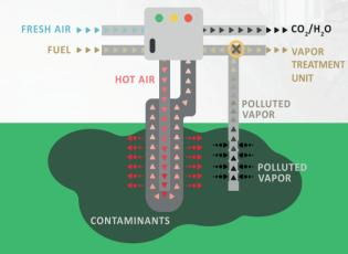
The **Smart Burners** technologies developed by Haemers Technologies have been especially designed to be quick, effective and applicable in complex environments while reducing the costs and environmenta impact of the thermal desorption process. They allow the contaminated soil to be heated in order to eliminate different kinds of pollutants: organic pollutants, hydrocarbons, chlorinated solvents, heavy metals (mercury), etc.
