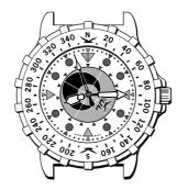
Advance just under three more days to day 6 at 8.15, and the CTD has moved on to show the next high at 10:10 and low at 16.15. The amount of water under the hour hand indicates half tide and rising.
