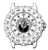
It is 10:10 on day 1. High tide was at 6.00. Observe where the hour hand cuts the tide graph to see there is less than half tide now, and the tide is going out. Low tide will be in two hours at 12:10
