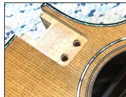
Bolt joint "double tenon" superior acoustic coupling, and ensure that fretboard stays straight
