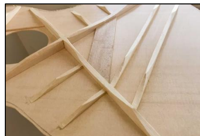
X-type bracing pattern (spruce)
