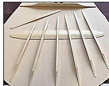
Lightweight fan bracing (spruce)
