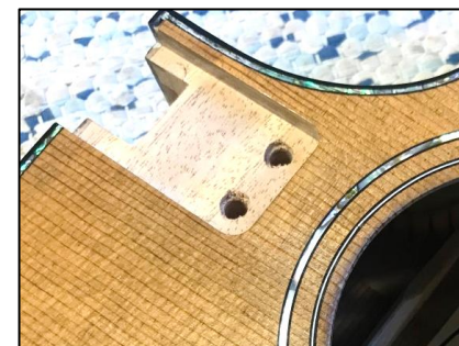
Bolt joint "double tenon" superior acoustic coupling, and ensure that fretboard stays straight
