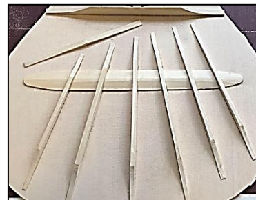
Lightweight fan bracing (spruce)
