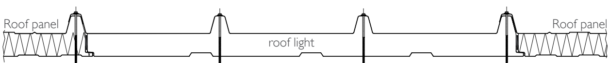
Cross section – installation/fastening through the foam core.
