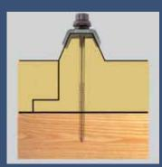
STRUCTURAL FIXING OF ROOF PANELS ON WOOD SUPPORT STRUCTURE FIXING
