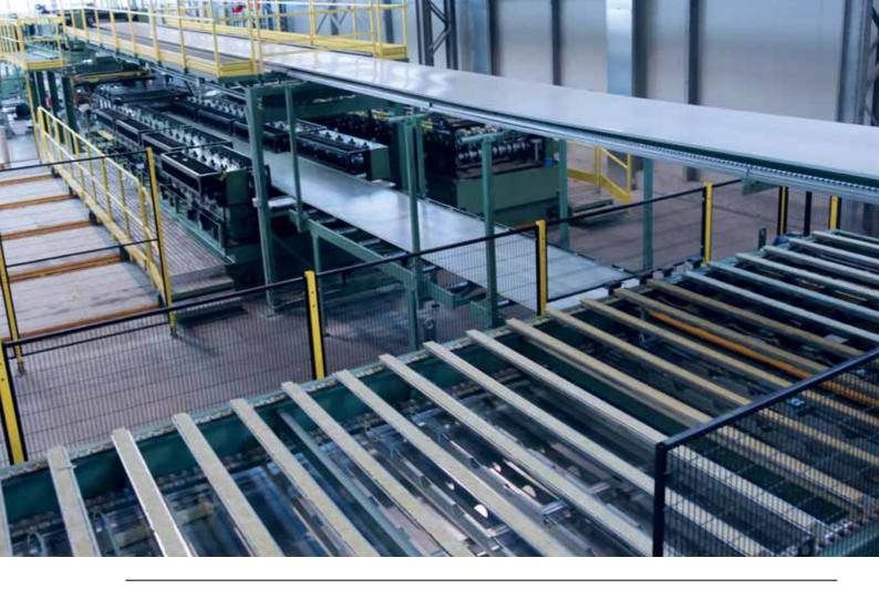
FROM PREPAINTED STEEL TO ZINC, COPPER OR ALUMINIUM.THE COATING OF THE PANEL IS ON DEMAND ACCORDING TO THE CLIENT'S REQUIREMENTS. AN IMPORTANT PRODUCTION LINE FOR A CONTINUOUS PROCESSING CYCLE THAT MAKES IT POSSIBLE FOR EACH ORDER TO BE MADE AD HOC. FROM THE STEEL COILS TO THE PACKAGING, EVERYTHING IS MADE BY MAINTAINING THE CONTINUOUS PRODUCTION PACE. THIS SEQUENCE OF PICTURES SHOWS THE
