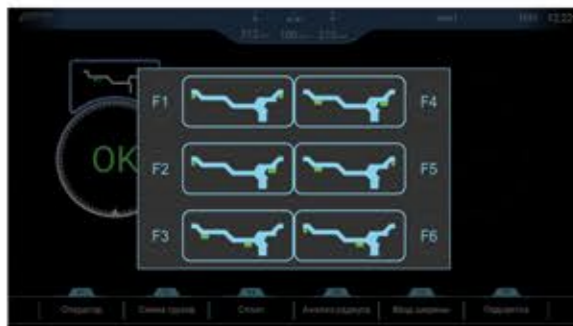
Balancing weight installation scheme selection
