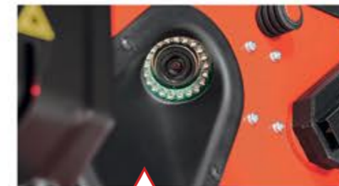
Laser 3D scanner Precisely scans the inner rim surface with specific profiles and automatically identifies the optimal points for weight installation
