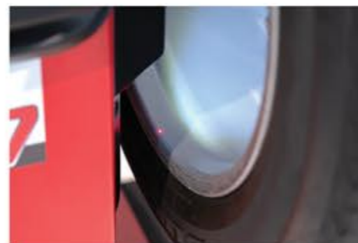
Laser pointer for precise pointing of adhesive weights installation place
