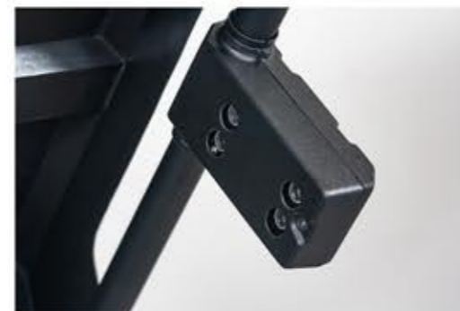
Ultrasonic sensor for recognition of weight installation coordinates on the outer rim surface
