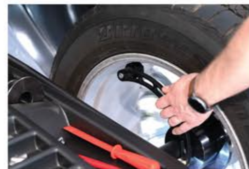
Electronic gauge allows automatic identification of the coordinates for balancing weight installation on the rim inner surface. Electronic gauge handle allowing precise alignment and installation of adhesive weights.
