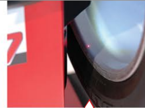
LP (laser pointer) Laser pointer for precise indication of the weight installation point
