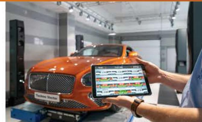
TechnoVector 8 Velox is recommended for installation in acceptance areas of car repair shops and dealership centers for quick and contactless wheel alignment check
