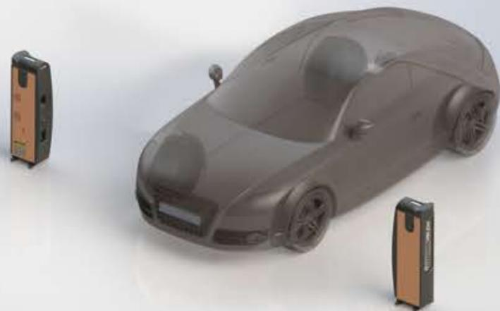
Sequential measurement of front and rear axle
