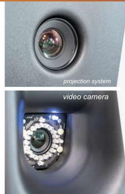
A contactless machine vision system
