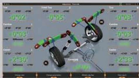
The TechnoVector 8 software is a powerful and modern means for checking and controlling wheel alignment
