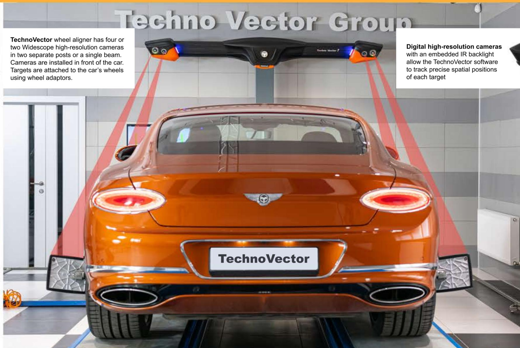
**TechnoVector** wheel aligner has four or two Widescope high-resolution cameras in two separate posts or a single beam. Cameras are installed in front of the car. Targets are attached to the car's wheels using wheel adaptors.
