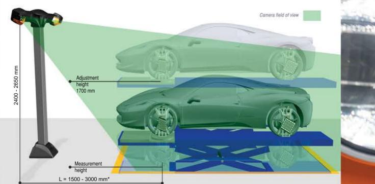
\* Visibility of targets at the lift floor level may be reached at the distance starting from 2200 mm
