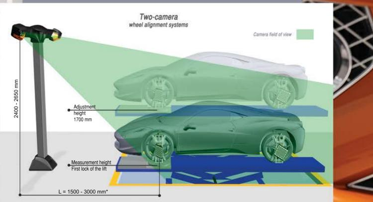
\* For the first stop of the lift targets fit into the field of view at approximately 2600 mm
