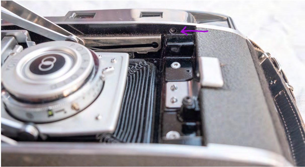
1 first screw, lens well Polaroid 110 A
