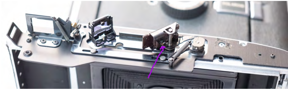
Polaroid 110A, rangefinder setup
