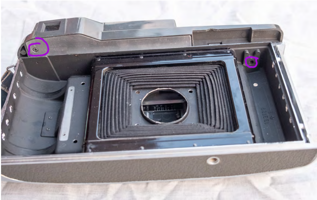
2 & 3 second and third screw, under finder window and center of take up spool
