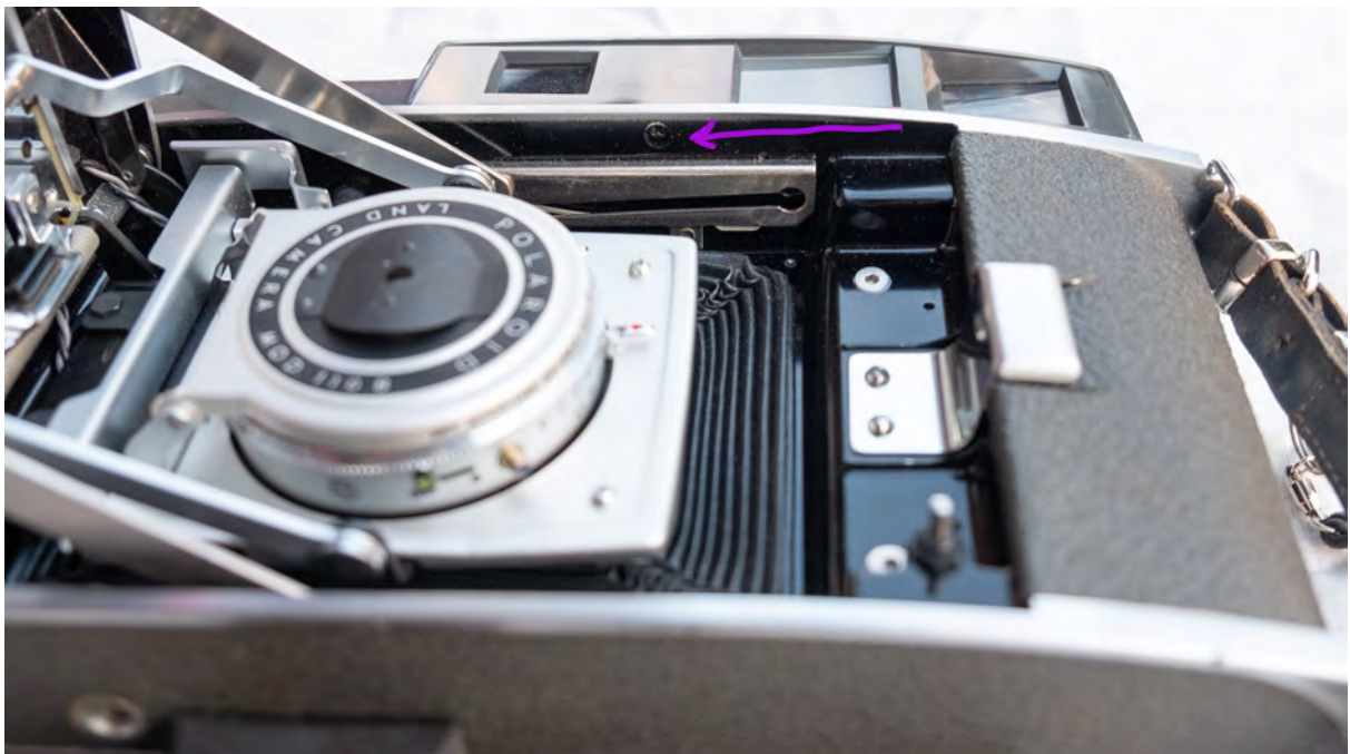
1 Screw lens well, Polaroid 110B, note the slightly different location from the 110A.
