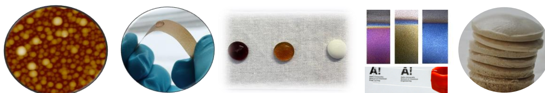
Figure 1. AFM image of LNPs, examples of strong, water-resistant nanocomposite, multifunctional textile coating, transparent or photonic colours and foams using LNPs.
