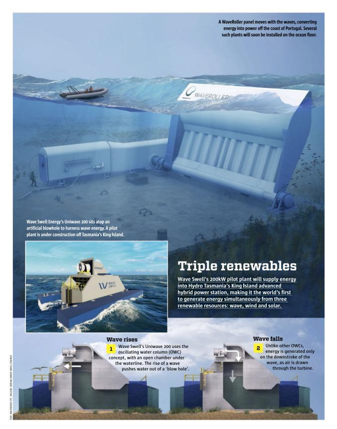
AW-Energy, which installs steel panels 10 to 20 metres under the water surface, a few hundred metres from the coast. A test plant off the Portuguese seaport of Peniche already generates 1MW for the city via this hydraulic system, and more WaveRollers will soon be tested in Mexico and South-East Asia.
