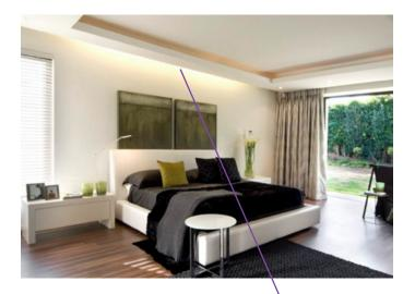
An LED strip can be used in a recess cut at the back of the bulkhead to give a subtle wash of light down the wall.
