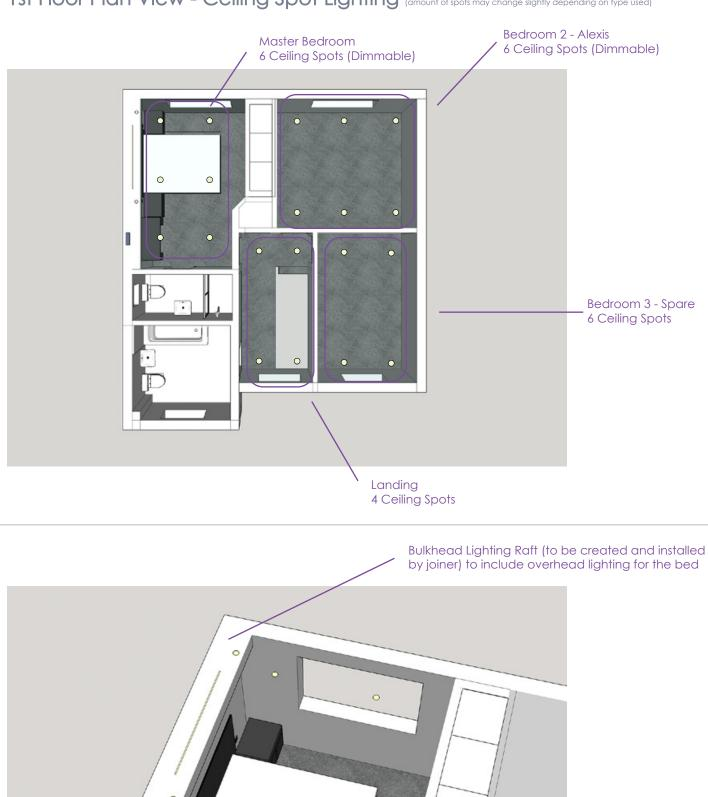
1st Floor Plan View - Ceiling Spot Lighting (amount of spots may change slightly depending on type used)
