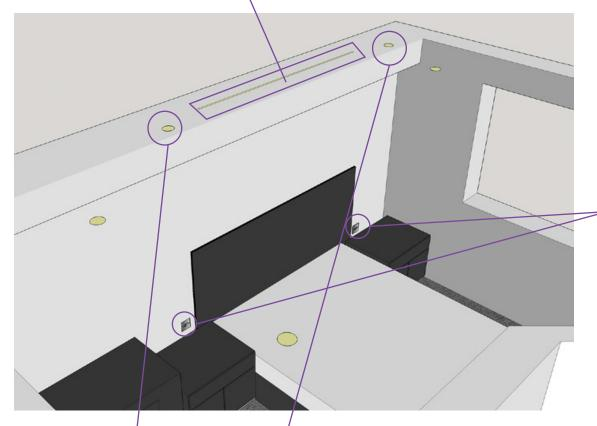
2 gang dimmer switches. One to control their corresponding spotlight and one each to control the LED strip.
