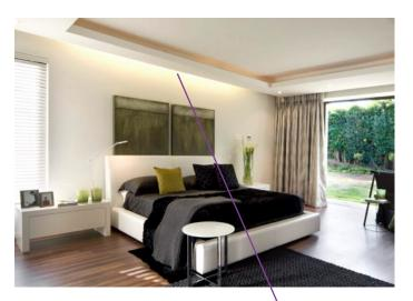
An LED strip can be used in a recess cut at the back of the bulkhead to give a subtle wash of light down the wall.
