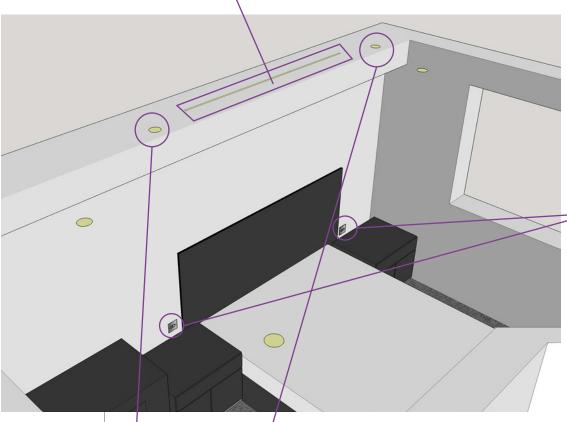
2 gang dimmer switches. One to control their corresponding spotlight and one each to control the LED strip.
