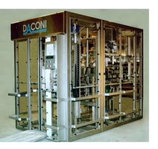
Complete Trolley filler line with Shrink Wrapper type SW2018 and Trolley Filler type TF2010
