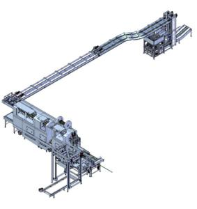
**BUFFER AND GROUPING PLATE BETWEEN WASHING AND PALLETIZING**
