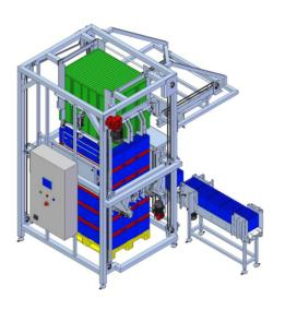
LIFTING SYSTEM AND GROUPING PLATE FOR PALLETIZING
