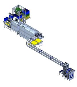
**BUFFERSYSTEM WITH MANUAL** IN/OUT-FEED OF EGG TRAYS
