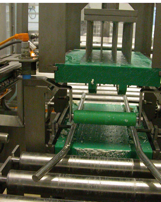
MULTISTEP PIERCING MACHINE FOR DIFFERENT CHEESE SHAPES
