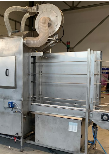
GUIDED INPUT SECTION BUILD IN BLOW DRYING SYSTEM
