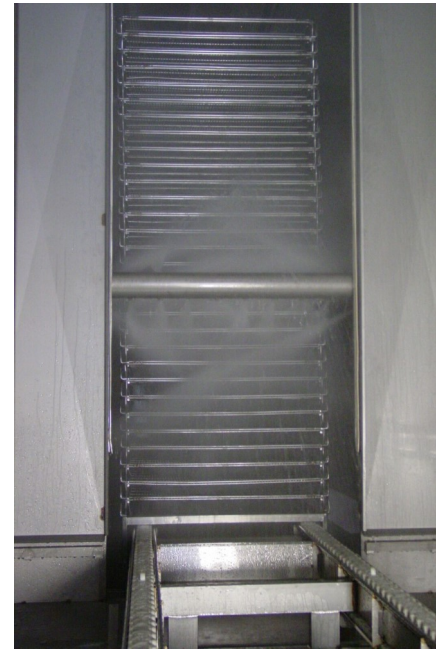
TROLLEY CLEANING WITH ONE WAY ENTRANCE
