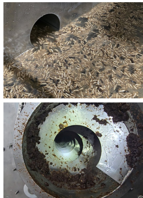
SOAKING BATH SYSTEM FRASS SEPARATION
