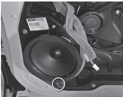
**Hint:** Don't forget to connect the tweeter cable (with crossover) to the OEM harness, before reassembling the door panel. The crossover needs to be placed behind the door panel. Use foam pads to wrap cables/crossover to prevent rattling.
