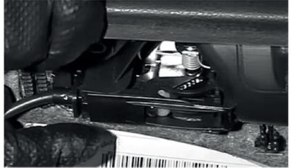
Disconnect all cables for lighting, speaker cable harness and any other connections.
