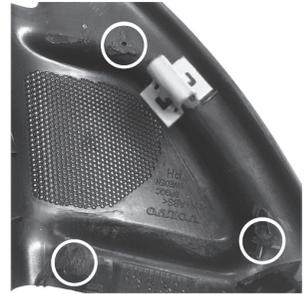
Attach the 3M double-sided adhesive tape to the sound optimized tweeter bracket. Mount the new DLS tweeter in the bracket. Remove the protection plastic from the 3M tape and place the bracket in the OEM tweeter cover. Press the bracket down, to attach to the OEM tweeter cover.
