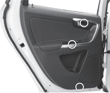
Be careful when removing the door panels and lids. Use PRY tools.
