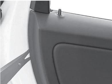
Some newer models don't have plastic clips to hold the door in place. Just remove the screws and gently press the door panel up. Be careful with the door lock knob. Just move the panel straight up.
