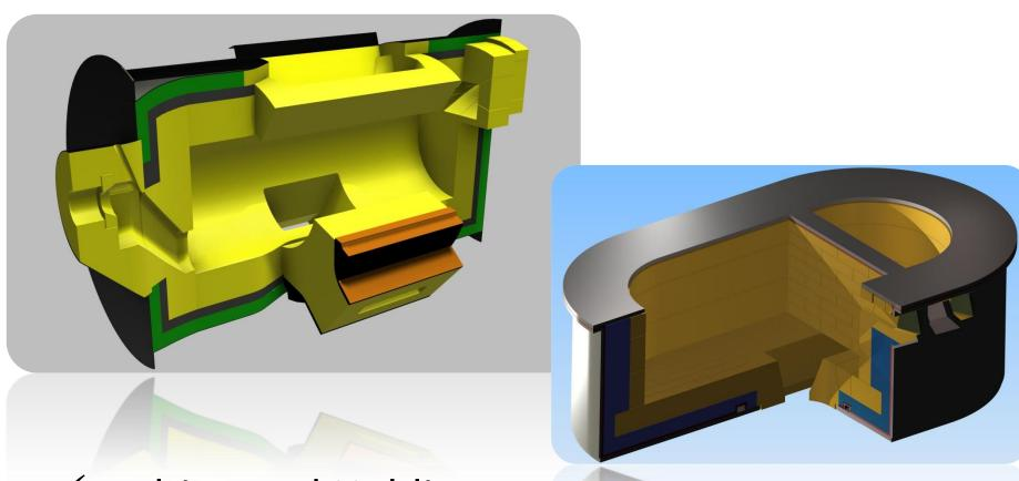
✓ Melting and Holding Furnace
