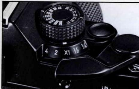
**7. Align the exposure compensation pointer with 'X1'**
