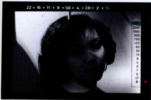
3. When the LED dot comes on in alignment with 'B' set the aperture ring to a wider lens opening. If the LED dot fails to move upward even at maximum aperture, resort to flash exposure.
