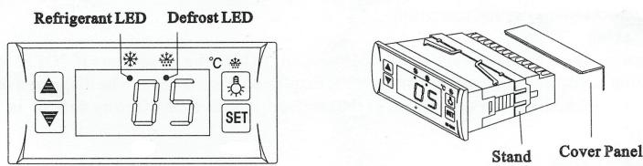
It is a mini-sized and integrated intelligent controller and applicable to the compressor of 1 HP.
