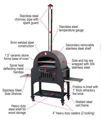
This medium wood burning oven is constructed from 6mm steel with black hi-heat resistant paint finish and a 304 stainless steel wrap, ensuring superior outdoor cooking function and enjoyment for many years.
