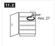
Insert the antenna and fasten it by tightening the nut with the wrench.
