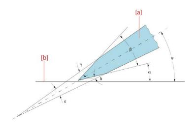
The knife/blade must never be placed on an angle that is too flat since the knife/blade does not cut into the block at all this way. Only the rear side slides over the sectioning surface.
