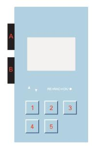
If knob [B] is kept at a high speed for more than two seconds, the specimen will automatically move to the rear position.
