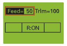
In the NORMAL display mode, an outline around the value is shown on the display.
