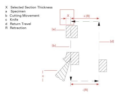
The yellow LED Retraction lights up. If desired, the function <retraction> can be turned off.
