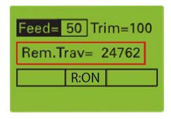
This value shows the distance in microns, which is left for sectioning in microns.
