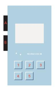
• To choose between section thickness and trimming thickness, press the knob [A]
