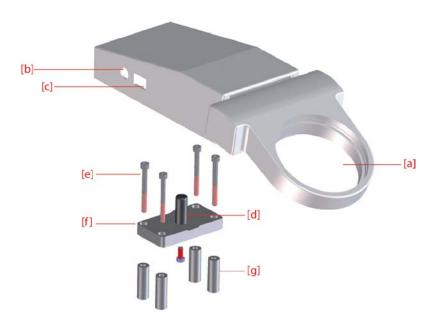
Connect the integrated light to the power outlet with the power cord [b] and turn it and off with the switch [c].
