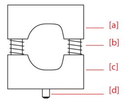
• The pin [d], which fits into the lower clamping jaws [c], positions the insert precisely. The two springs [b] help to remove the speci- men from the inserts.
