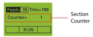
The section counter adds up the number of sections produced. After each downward movement of the specimen holder, the number on the section counter increases by 1.
