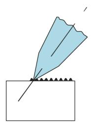
Between these two limit cases, the correct knife angle must be determined. A clearance angle between facet angle and block surface of approx. 5° is normal.
