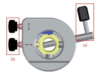
To bring the specimen into the desired position, move the clamping lever [a] towards the front.
