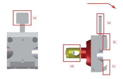
• To insert or remove the cassette from between the fixed [b] and movable [c] jaws, pull the lever [a] to the front (in the direction of the arrow).
