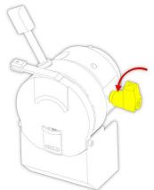
• Loosen the specimen head clamping lever to allow adjustment of the specimen parallel to the cutting edge.
