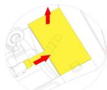
Remove the Vacutome hose and lift off the cover.
