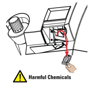
• Dispose of the used Purge Tray according to local regulations.
