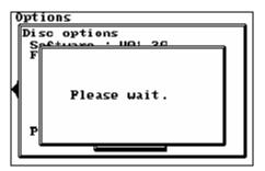
When the Wait screen has gone and the light on the USB Disk Drive Emulator has gone out, it is safe to remove the memory stick from the USB Disk Drive Emulator.
