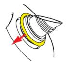
C: Allow the O-Ring seal to snap into place, then ensure it is properly seated in the Recess.
