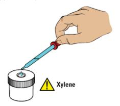
• Use the end of the pipette to push the central well down, to ensure that the Xylene levels are consistent.
