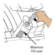
Replace the Mountant bottle cap and twist clockwise by hand to tighten it.
