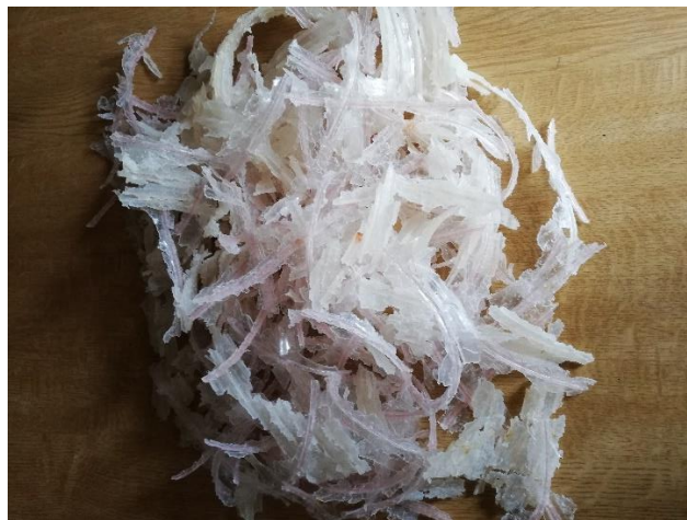
Recovered PU just after the jetting.
