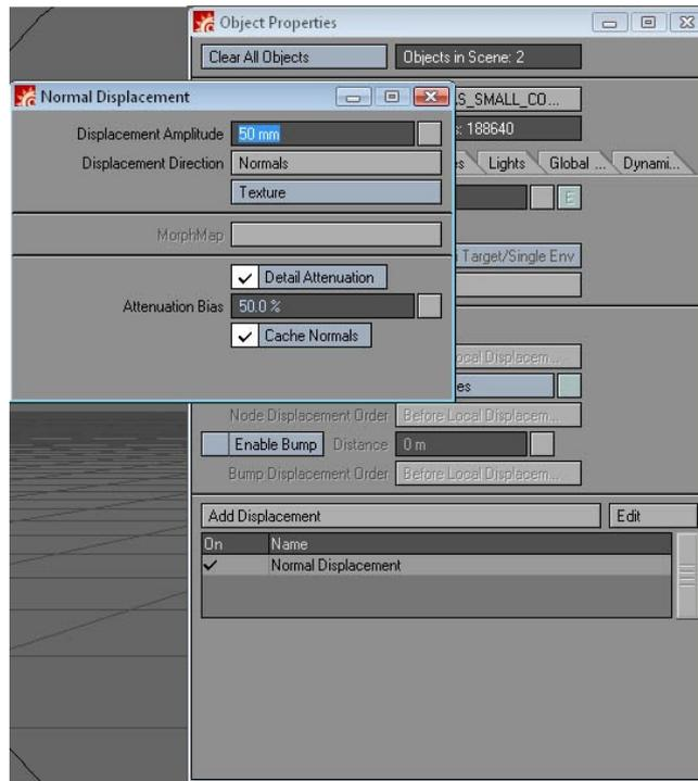
*Set the Displacement Amplitude to 50mm.*
