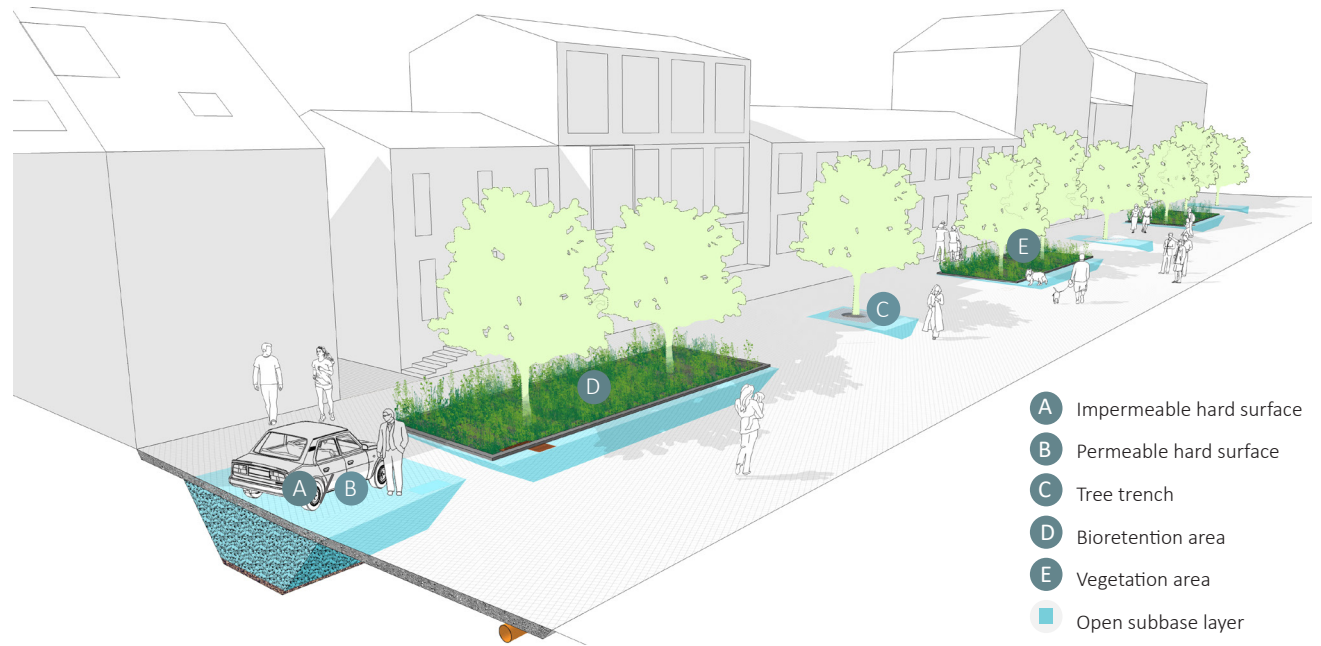
Figure 14. Example of a street with a BGG system made up of separate structures. Areas marked blue are individual sections of open subbase layer. These are laid separately under ground level structures such as bioretention areas, vegetation areas and tree trenches. The choice of structure installed is up to the designer which gives the BGG system flexibility. The open subbase layer contributes with gas exchange and water treatment or storage to a limited extent.
