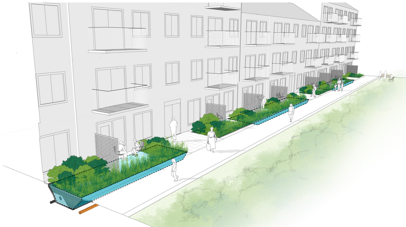
Figure 52. Illustration of individual constructions with an open subbase layer along the house facade and courtyard street.
