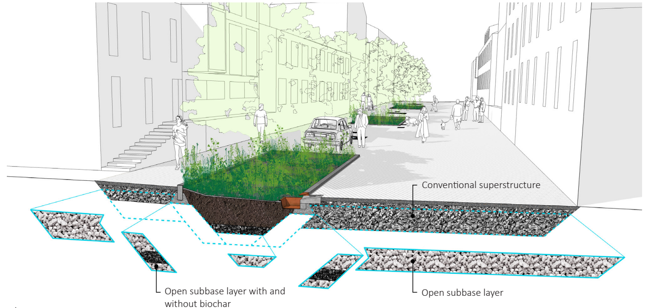
Figure 18. Open subbase layer can be expanded under pedestrian and bicycle paths and traffic lanes to increase the amount stormwater handled and the size of planting beds. Being able to determine the size and placement of open subbase layer makes it easier to combine the BGG system with other types of ground construction as well as meet future design needs and wants.
