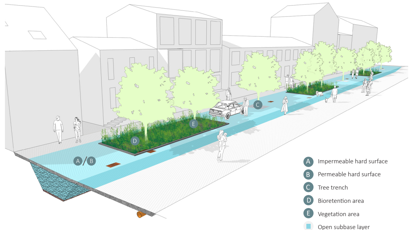
Figure 5. Example of an urban street with BGG located in the flex zone. The blue area symbolizes an open subbase layer which lies alongside the entire street. Hard surfaces with bioretention areas, green space and trees are alternated at will. Stormwater can be handled in a variety of ways while at the same time allowing flexibility in the design of street.
