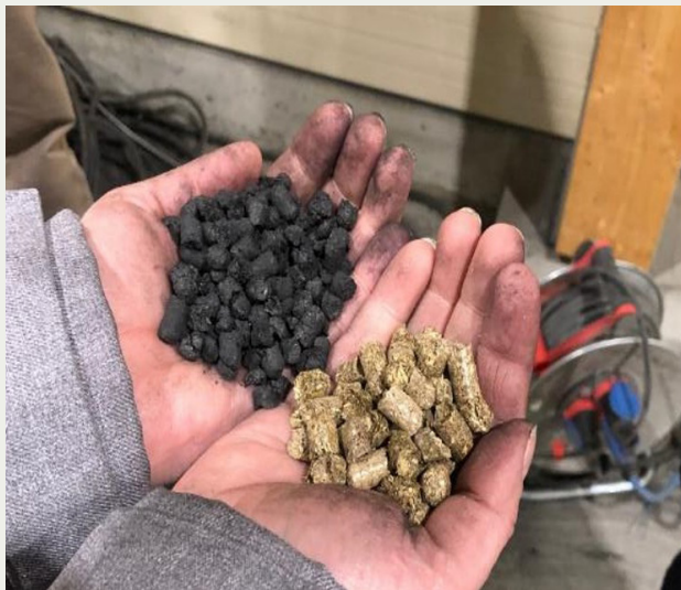
The left hand is holding biochar which has undergone pyrolysis. In the right is the raw material, in this case pellets of surplus organic material.
