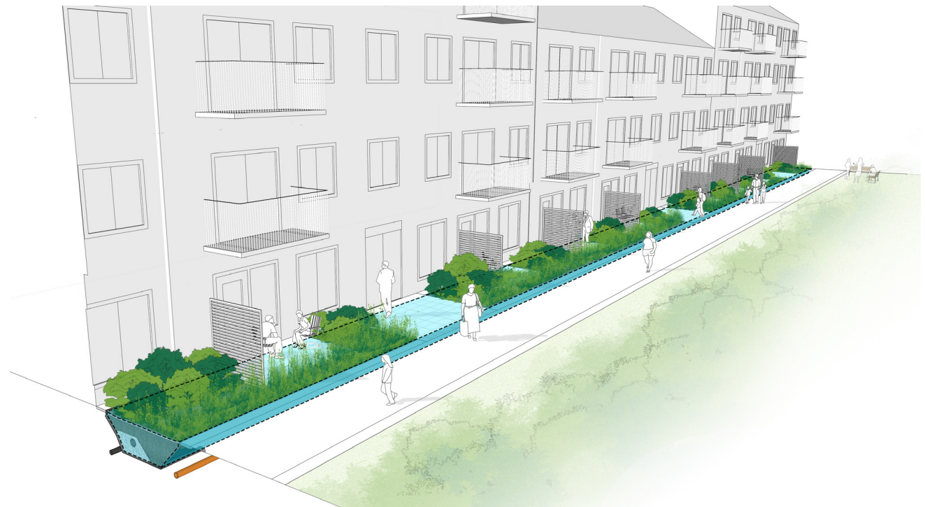
Figure 51. Illustration of a continuous stripe with an open subbase layer along the house facade and courtyard street.
