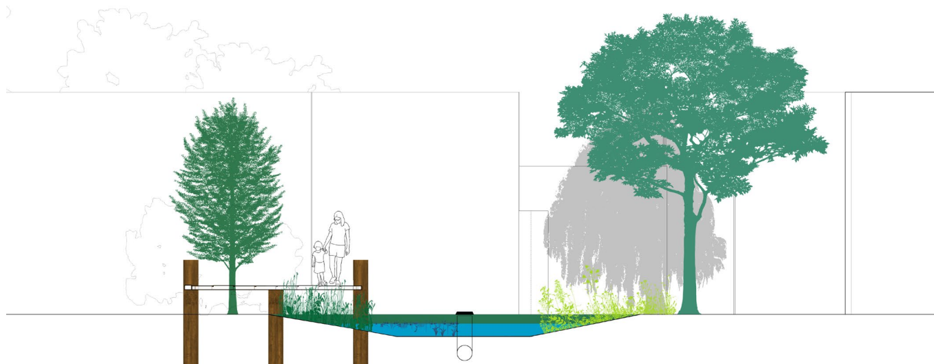
Figure 108 - section of suggested semi-private wet basin with an outlet, which would allow discharge of rain water into cloudburst pipe during periods of heavy rain
