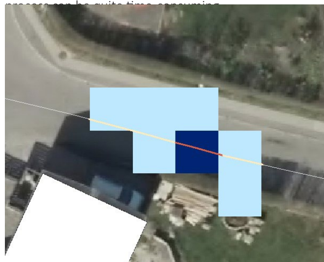
Figure 44 – Node where dark blue pixel represents water that is higher than 30 cm. The pixel does not cover the whole width of the street; therefore it is not the real thread for the traffic. However, because it is located directly on the polyline, the programme would recognize it as inaccessible.
