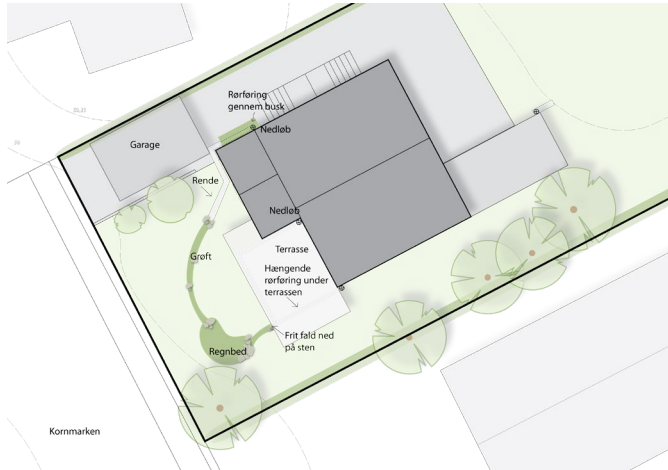
Figure 32 - a private garden that uses a gully, a bioswale and one big rain garden to handle rain water
