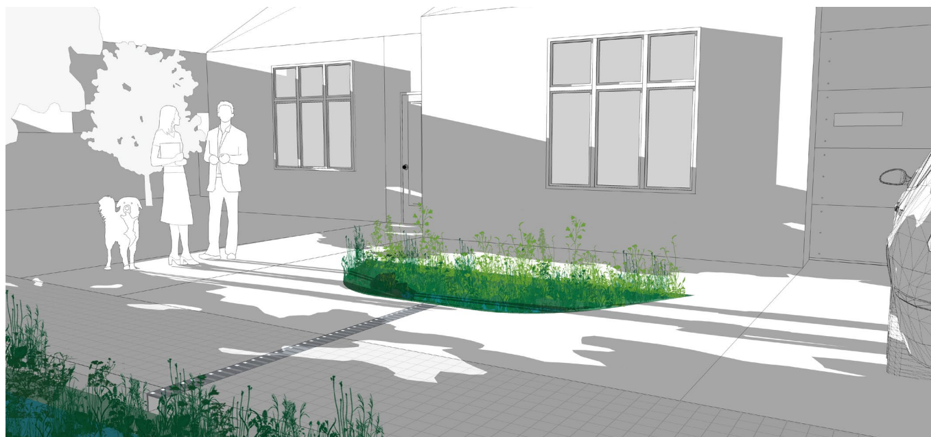
Figure 104 – Existing downpipe could be disconnected at the bottom of the building and rainwater could be led through terrain to the newly-established rain garden. The rainwater from the rain garden would be discharged through existing storm water pipe into the nearest public BGI feature. During extreme rain, it could overflow through terrain and trench, which would be under a sidewalk into the nearest BGI feature on the street.
