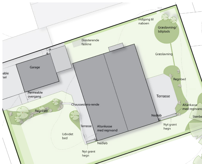
Figure 36 - another private garden with diverse BGI solutions that consists of two rain gardens, gullies, storm water planters and small dry basin
