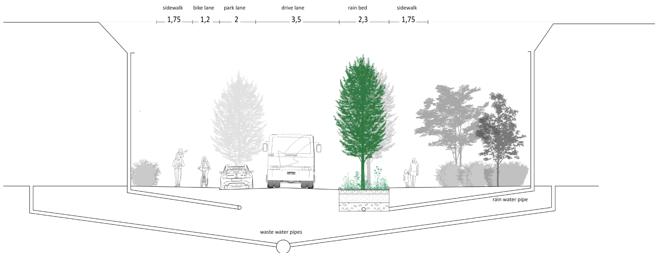
Figure 89 – section of 12,5-meter street – This street typology, in addition to a 10-meter street, contains bus traffic and cycle traffic. Width of all functions on this street compare to a 10-meter street is extended but width of parking lanes stays the same. The enlargement is particularly necessary for passing points and a drive lane that contains the minimal width for bus traffic. The length of passing points was increased up to 15 meters.
