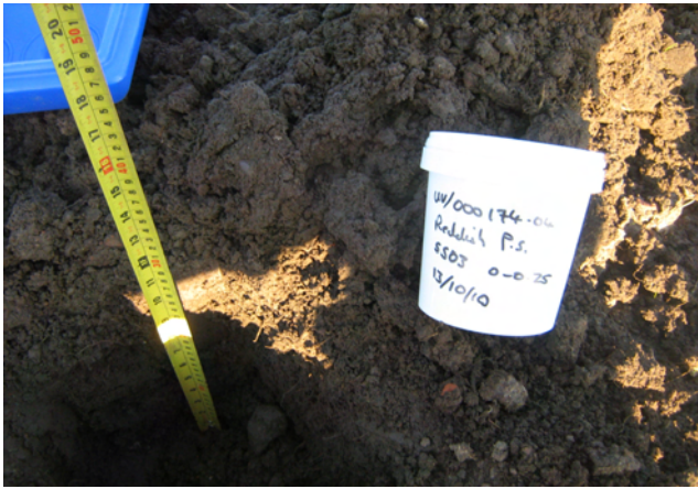
1. SS03 verification of subsoil depth - 250mm deep
